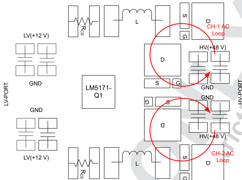
8-24. A Layout Example of Dual-Channel Power Circuit Placement
