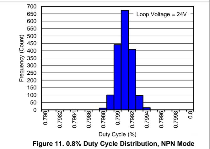
Figure 11. 0.8% Duty Cycle Distribution, NPN Mode
