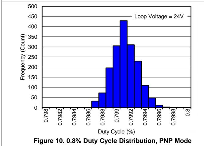
Figure 10. 0.8% Duty Cycle Distribution, PNP Mode
