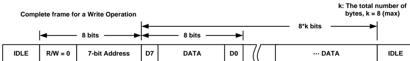
Figure 16. Complete Frame For A Write Command
