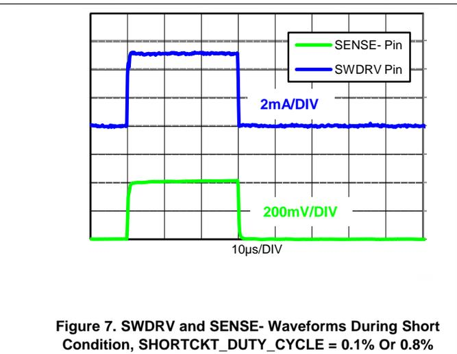
Figure 7. SWDRV and SENSE- Waveforms During Short Condition, SHORTCKT\_DUTY\_CYCLE = 0.1% Or 0.8%
