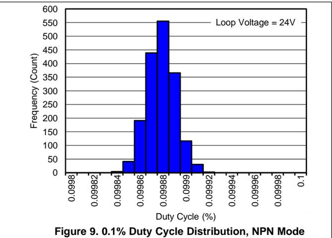
Figure 9. 0.1% Duty Cycle Distribution, NPN Mode
