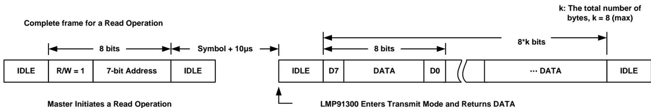
**Figure 18. Complete Frame For A Read Command**
