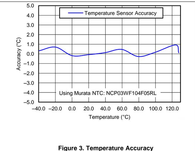
Figure 3. Temperature Accuracy
