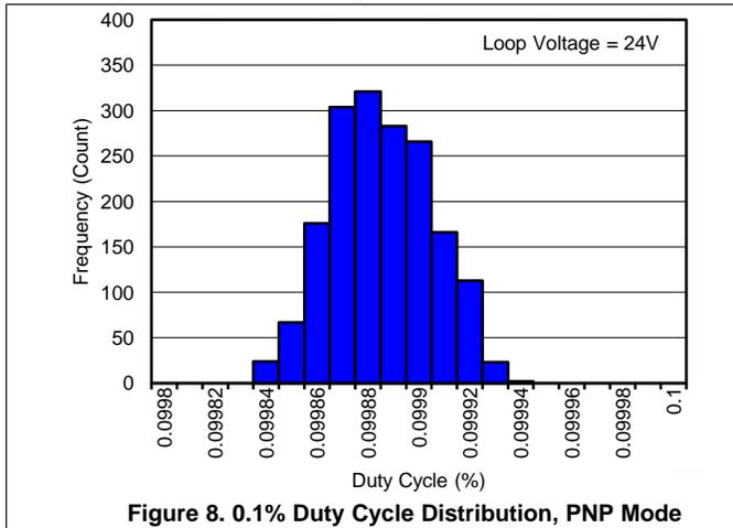
Figure 8. 0.1% Duty Cycle Distribution, PNP Mode
