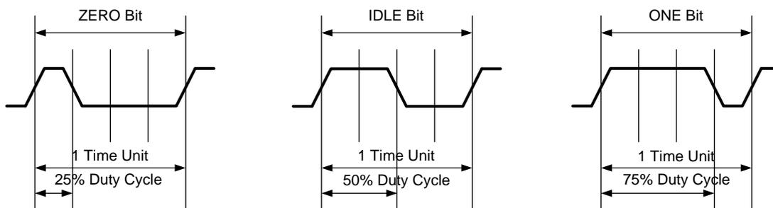
Figure 15. Single Wire Interface (SWIF) Symbol Diagram
