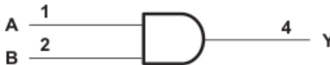
図 7-1. Logic Diagram (Positive Side)
