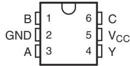
☒ 4-1. DBV OR DCK Package 6-Pin SOT-23 or SC70 Top View
