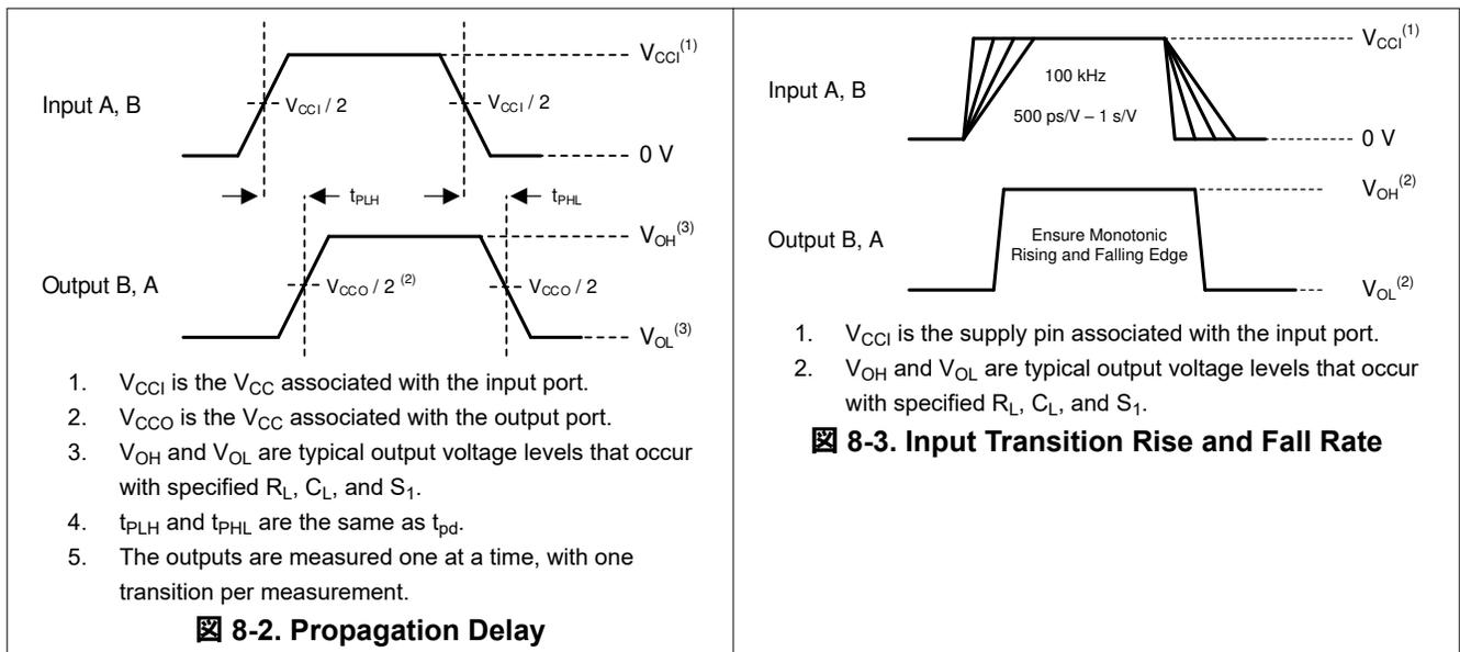
图 8-3. Input Transition Rise and Fall Rate
