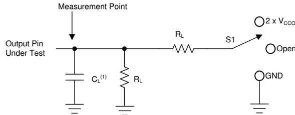
A.  $C_L$  includes probe and jig capacitance.
