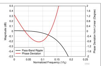
図 8-62. Ultra-Low-Latency Decimation Filter Pass-Band Ripple and Phase Deviation
