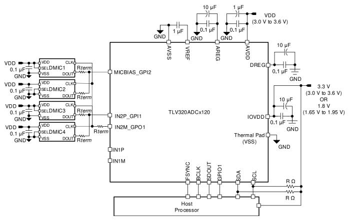
図 9-4. Four-Channel Digital PDM Microphone Recording Diagram
