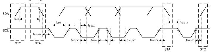
図 7-1. I<sup>2</sup>C Interface Timing Diagram
