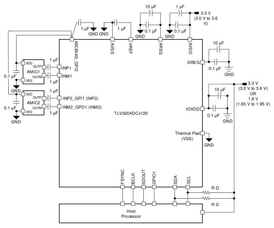
図 9-1. Two-Channel Analog Microphone Recording Diagram
