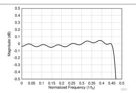
図 8-26. Linear Phase Decimation Filter Pass-Band Ripple
