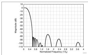
図 8-35. Linear Phase Decimation Filter Magnitude Response
