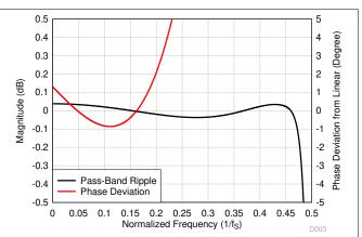
図 8-58. Ultra-Low-Latency Decimation Filter Pass-Band Ripple and Phase Deviation
