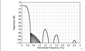
**図 8-33. Linear Phase Decimation Filter Magnitude**Response
