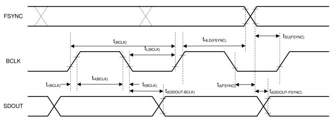
図 7-2. TDM (With BCLK\_POL = 1), I<sup>2</sup>S, and LJ Interface Timing Diagram
