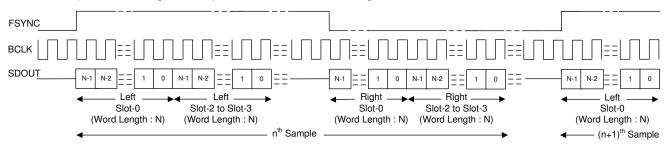
図 8-9. LJ Mode Standard Protocol Timing (TX\_OFFSET = 0)
