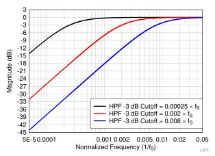
図 8-17. HPF Filter Frequency Response Plot
