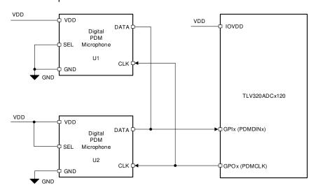
図 8-64. Digital PDM Microphones Connection Diagram for the TLV320ADC3120
