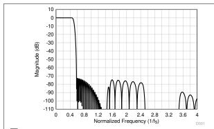
図 8-19. Linear Phase Decimation Filter Magnitude Response
