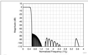
**図 8-29. Linear Phase Decimation Filter Magnitude**Response
