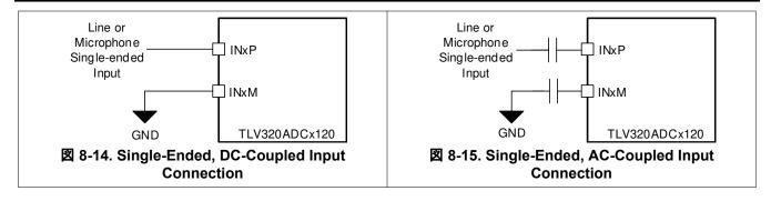
The device allows for flexibility in choosing the typical input impedance on INxP or INxM from 2.5 k $\Omega$  (default), 10 k $\Omega$ , and 20 k $\Omega$  based on the input source impedance. The higher input impedance results in slightly higher noise or lower dynamic range.  $\frac{1}{8}$  8-9 lists the configuration register settings for the input impedance for the record channel.
