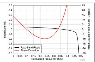
図 8-50. Ultra-Low-Latency Decimation Filter Pass-Band Ripple and Phase Deviation
