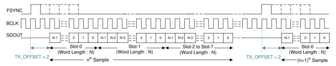
図 8-2. TDM Mode Protocol Timing (TX\_OFFSET = 2)
