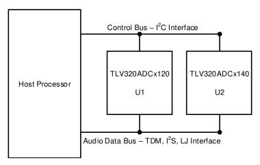
図 8-13. Multiple Devices With Shared Control and Audio Data Buses
