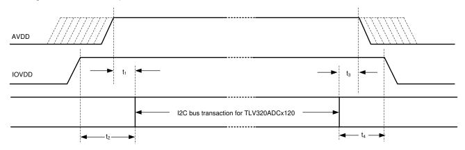
図 10-1. Power-Supply Sequencing Requirement Timing Diagram
