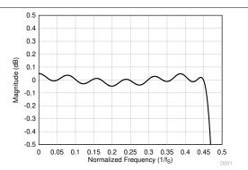
図 8-30. Linear Phase Decimation Filter Pass-Band Ripple
