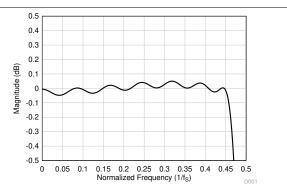
図 8-22. Linear Phase Decimation Filter Pass-Band Ripple
