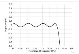
図 8-32. Linear Phase Decimation Filter Pass-Band Ripple
