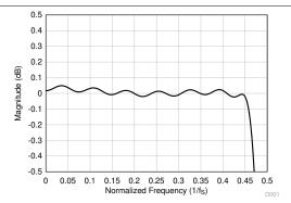
図 8-20. Linear Phase Decimation Filter Pass-Band Ripple
