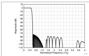
図 8-23. Linear Phase Decimation Filter Magnitude Response
