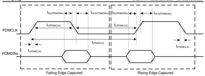
図 7-3. PDM Digital Microphone Interface Timing Diagram
