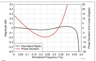
図 8-54. Ultra-Low-Latency Decimation Filter Pass-Band Ripple and Phase Deviation
