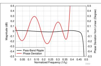
図 8-44. Low-Latency Decimation Filter Pass-Band Ripple and Phase Deviation
