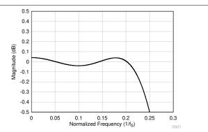
図 8-34. Linear Phase Decimation Filter Pass-Band Ripple
