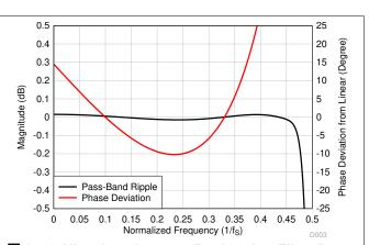
図 8-56. Ultra-Low-Latency Decimation Filter Pass-Band Ripple and Phase Deviation
