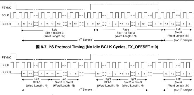
図 8-8.  $I^2$ S Protocol Timing (TX\_OFFSET = 0 and BCLK\_POL = 1)
