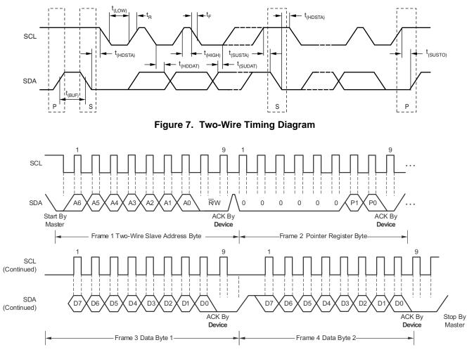
Figure 8. Two-Wire Timing Diagram for TMP275-Q1 Write Word Format
