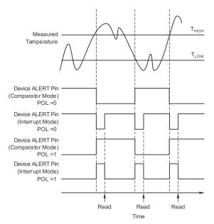
Figure 12. Output Transfer Function Diagrams
