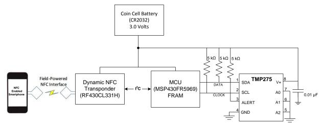
Figure 16. Temperature Data Logger
