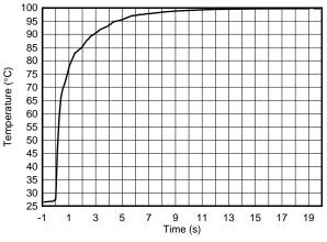
Figure 14. Temperature Step Response
