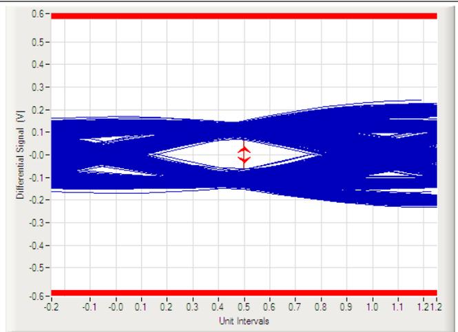
Figure 16. USB 3.1 Gen 2 10-Gbps Eye Diagram (with TPD1E01B04DPL)
