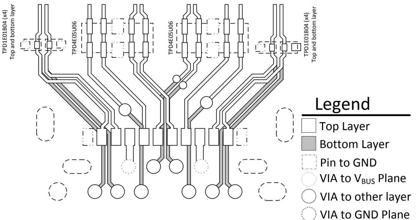
Figure 18. USB Type-C Mid-Mount, Hybrid Connector ESD Layout
