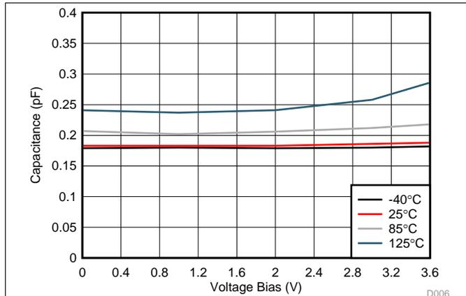
Figure 7. Capacitance vs. Bias Voltage (DPY Package)
