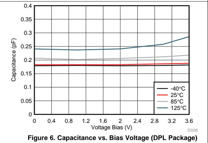
Figure 6. Capacitance vs. Bias Voltage (DPL Package)
