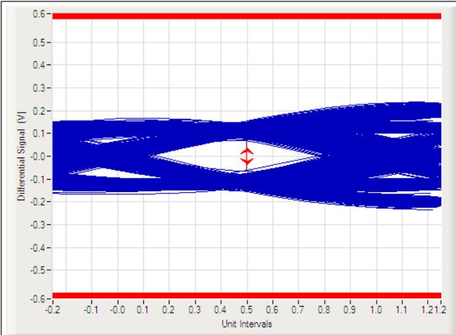
Figure 15. USB 3.1 Gen 2 10-Gbps Eye Diagram (Bare Board)
