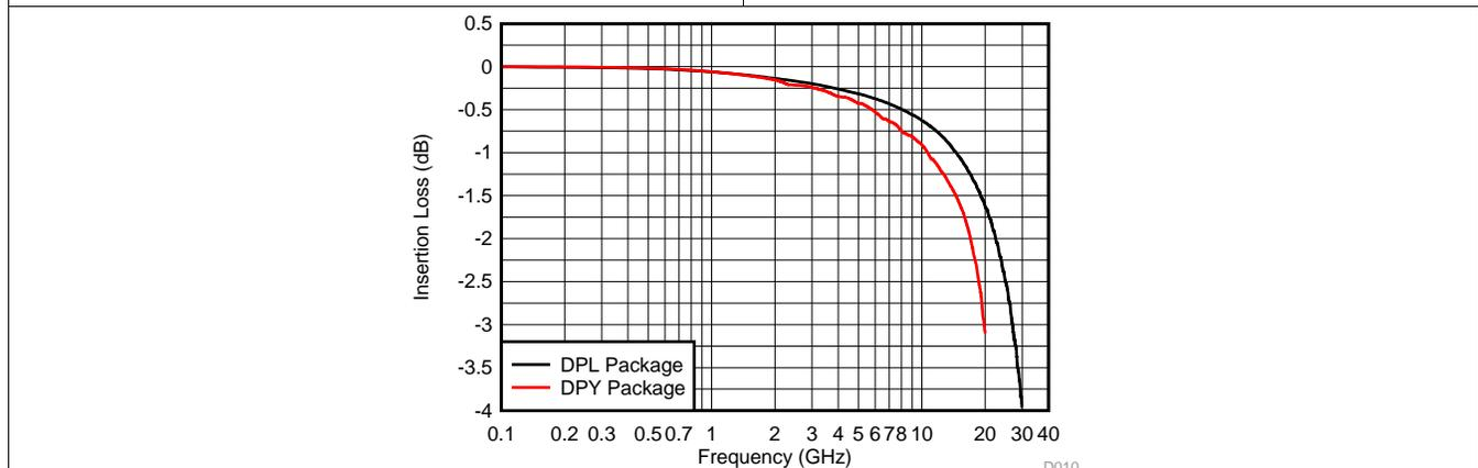
Figure 11. Insertion Loss
