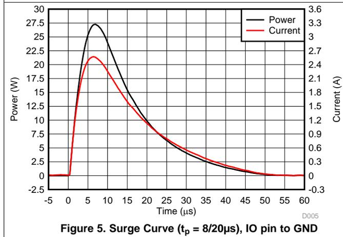
Figure 5. Surge Curve ( $t_p = 8/20\mu s$ ), IO pin to GND
