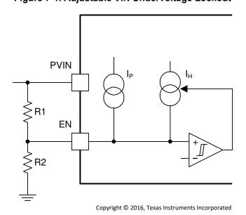
Figure 7-2. Adjustable PVIN Undervoltage Lockout, VIN ≥ 4.5 V
