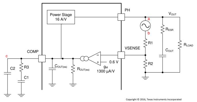
Figure 7-4. Small Signal Model for Loop Response
