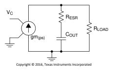
Figure 7-5. Simplified Small Signal Model for Peak Current Mode Control
