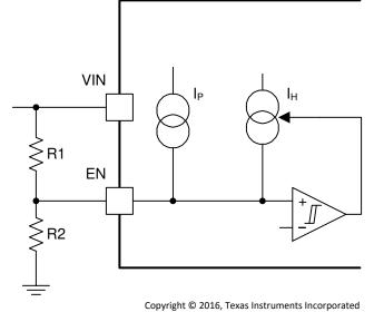
Figure 7-1. Adjustable VIN Undervoltage Lockout
