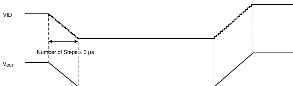
FIG 8-19. DVS Timing Diagram I (BUCKx_DECAY = 0)
