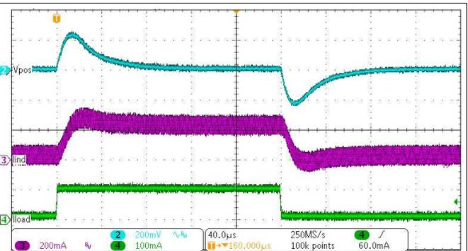
Figure 22. Inverting Buck-Boost Converter Load Transient Response
