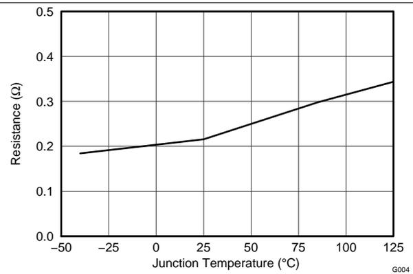
Figure 4. Inverting Buck-Boost Converter Switch  $r_{DS(on)}$
