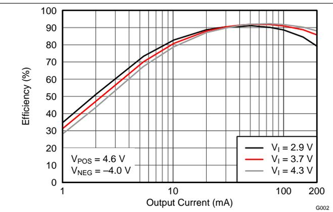
Figure 10. Efficiency vs. Output Current (Log Scale)
