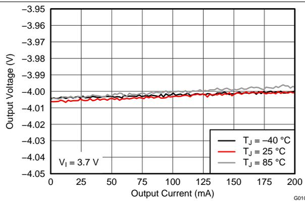
Figure 19. Inverting Buck-Boost Converter Load Regulation
