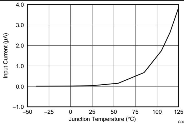
Figure 1. Shutdown Current into AVIN and PVIN
