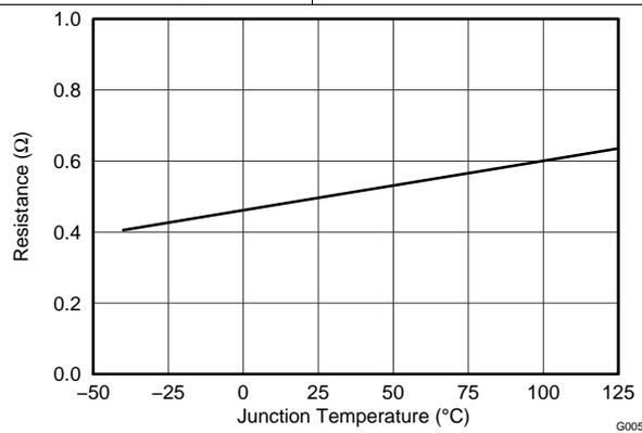
Figure 5. Inverting Buck-Boost Converter Rectifier  $r_{DS(on)}$
