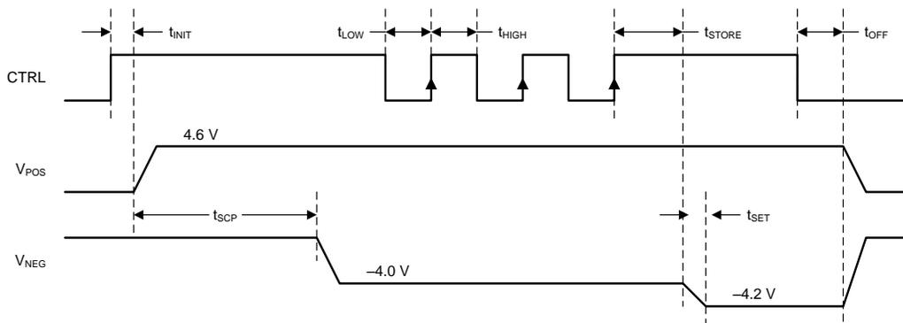
**Figure 7. Programming  $V_{NEG}$  Using the CTRL Pin**
