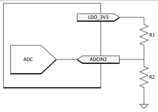
図 8-28. I<sup>2</sup>C Address Divider
