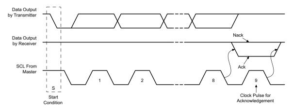
図 8-24. I<sup>2</sup>C Acknowledgment
