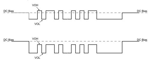
図 8-6. TX Driver Transmission with DC Bias
