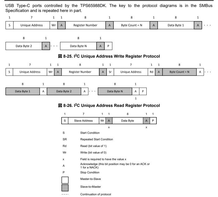
図 8-27. I<sup>2</sup>C Read/Write Protocol Key
