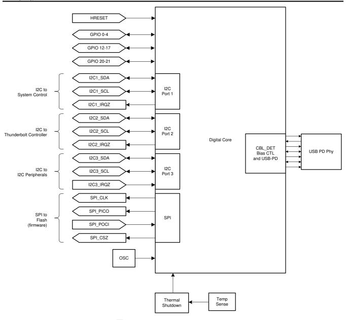
図 8-21. Digital Core Block Diagram
