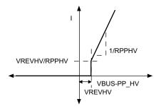
図 8-12. Ideal Diode Mode (Sink) Internal HV Switch I-V Curve
