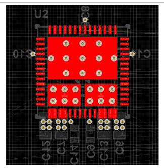
図 11-10. System Capacitors Placement Top Layer
