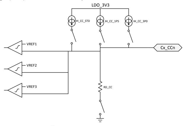
図 8-14. Plug and Orientation Detection Block
