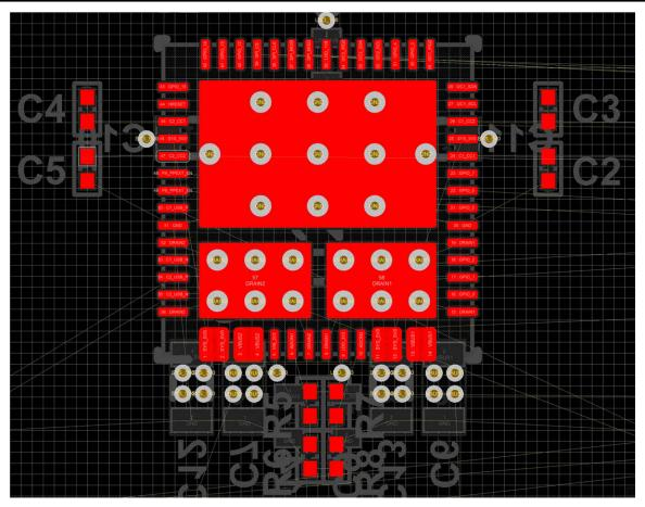
図 11-12. CC and ADCIN1/2 Component Placements
