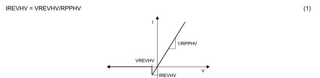
図 8-11. Comparator Mode (Source) Internal HV Switch I-V Curve
