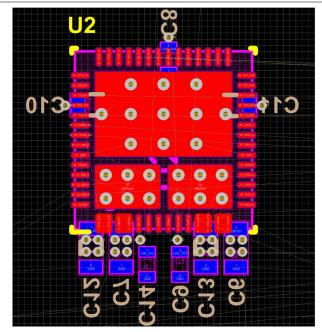
図 11-9. System Capacitors Placement Top/Bottom Layer
