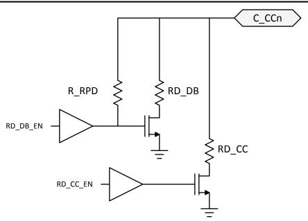
図 8-16. Dead Battery Pull-Down Resistor
