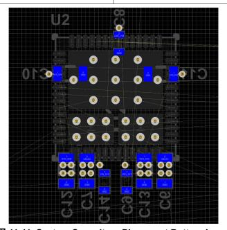
図 11-11. System Capacitors Placement Bottom Layer
