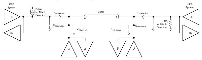
図 8-8. Example USB-PD Multi-Drop Configuration
