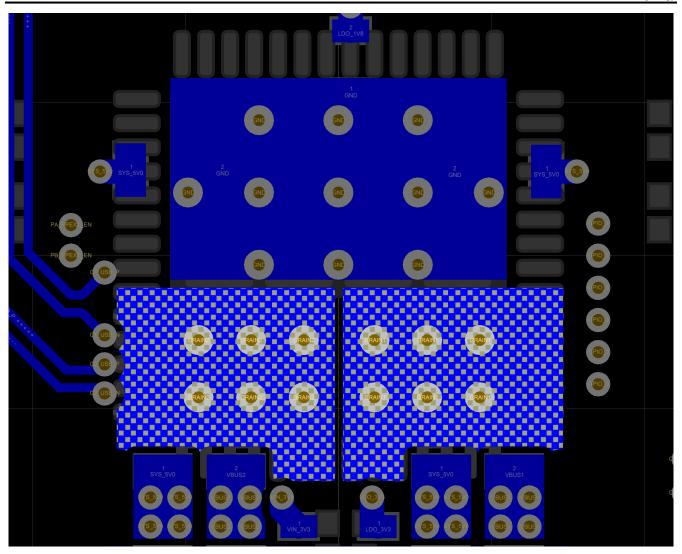
図 11-16. Figure 13. DRAIN1 and DRAIN2 Bottom Layer
