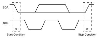
図 8-22. I<sup>2</sup>C Definition of Start and Stop Conditions
