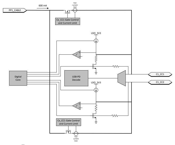
図 8-1. USB-PD Physical Layer, Simplified Plug and Orientation Detection Circuitry
