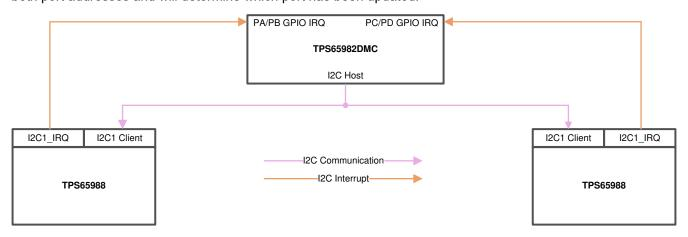
図 9-4. Interupt Configuration for DMC
