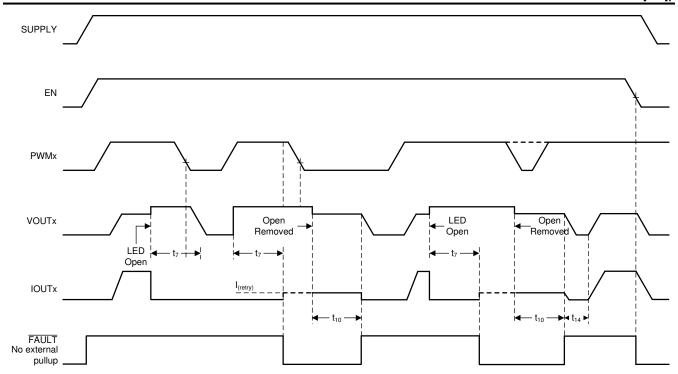
図 7-8. LED Open-Circuit Detection and Recovery Timing Diagram
