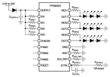
\*: 10nF ceramic capacitor is recommended for each OUTx to GND
