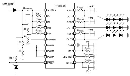
図 8-1. Typical Application Schematic
