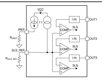
図 7-9. Single LED Short-Circuit Detection Block Diagram
