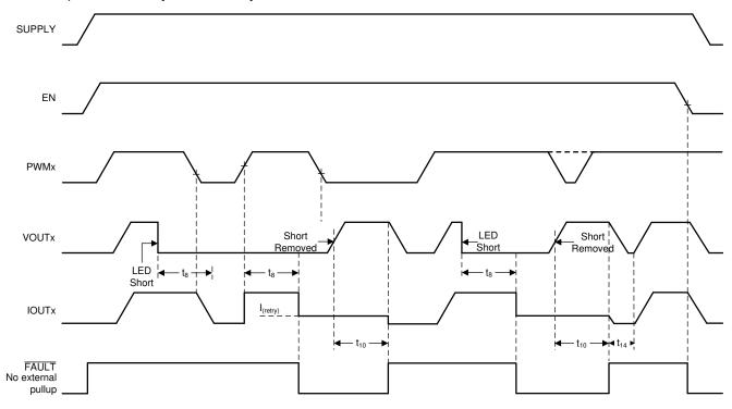
図 7-7. LED Short-to-GND Detection and Recovery Timing Diagram
