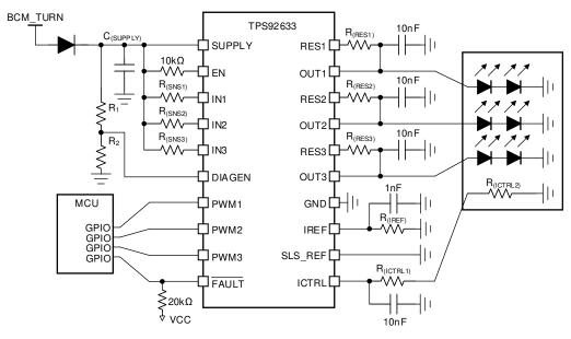
図 8-4. Typical Application Schematic
