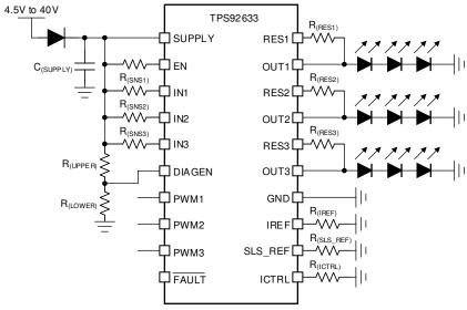
\*: 10nF ceramic capacitor is recommended for each OUTx to GND
