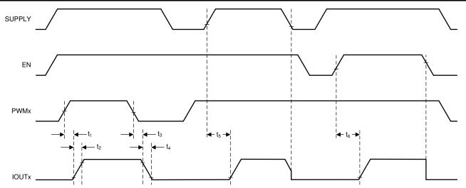
図 7-5. Power On Sequency and PWM Dimming Timing
