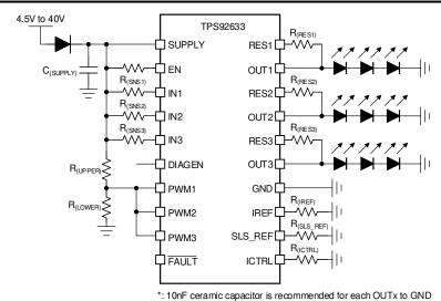
図 7-6. Application Schematic for Supply Control LED Brightness
