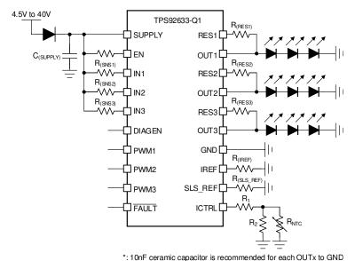
図 7-2. Application Schematic for External NTC Thermistor
