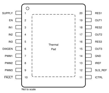
図 5-1. PWP Package 20-Pin HTSSOP With PowerPAD™ Package Top View
