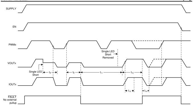
図 7-10. Single LED Short-Circuit Detection and Recovery Timing Diagram
