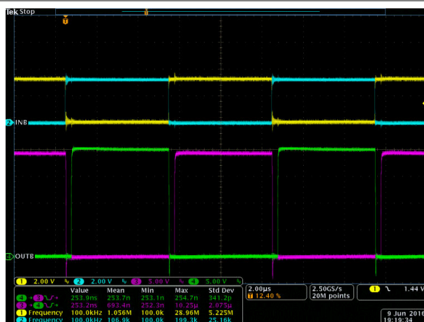
Figure 10-5. Bench Test Waveform for INA/B and OUTA/B
