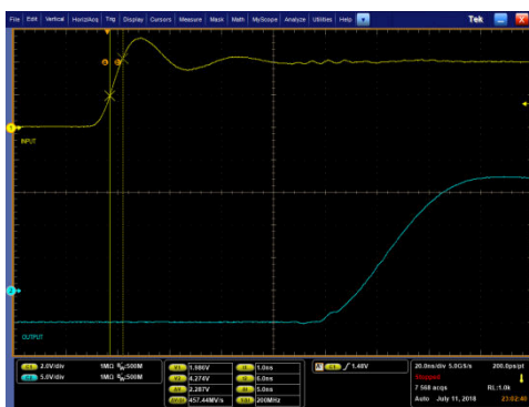
図 8-12. PWM Input (yellow) and Driver Output (blue) Rising Edge
