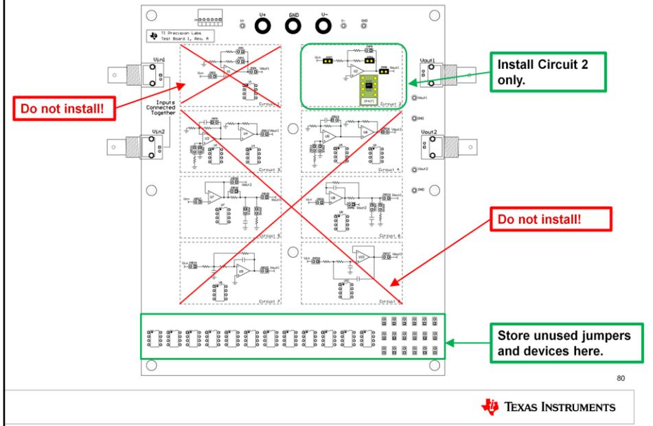
For this measurement, only circuit 2 is used. Do not install any jumpers or devices in any other circuits on the PCB! Remove any jumpers or devices from the unused circuits and store them in the storage area at the bottom of the test board.
