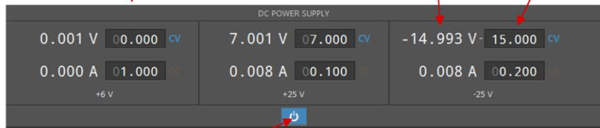
Press the power button to turn on the power supplies
