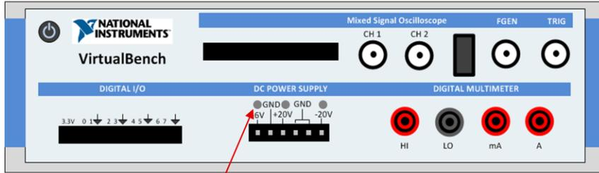
LEDs OFF = DC power supply OFF
