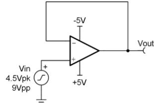
With a 9Vpp (4.5Vpk) input signal, is the circuit limitation caused by input common mode range or output voltage swing?
