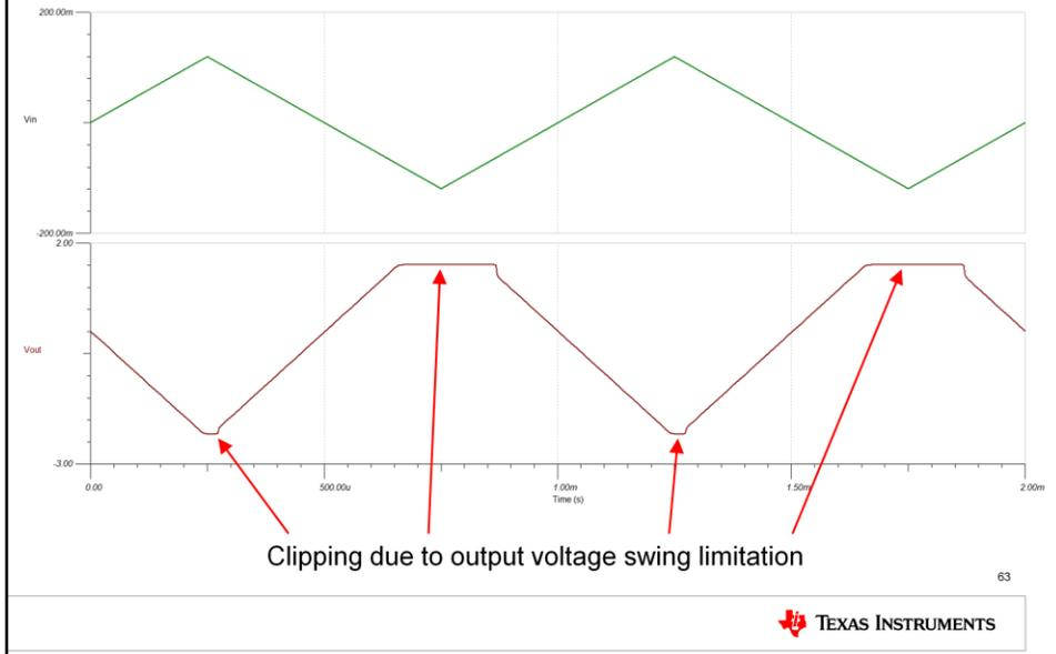
You should see a result similar to this.  $V_{in}$  is a triangle wave, as expected, but  $V_{out}$  clips at both the positive and negative ends of the triangle wave due to output voltage swing limitations.
