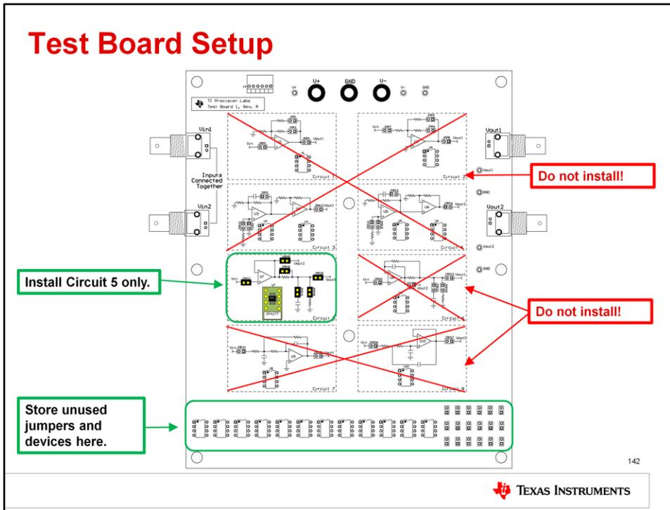
For the test board to function properly, it is important that you only install jumpers and devices in circuit 5. Do not install any jumpers or devices in any other circuits on the PCB! Remove any jumpers or devices from the unused circuits and store them in the storage area at the bottom of the test board.
