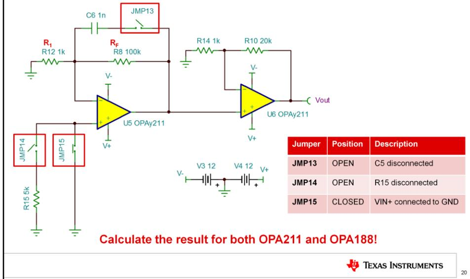
First, calculate the expected total output voltage due to  $V_{OS}$  and  $I_B$  for the circuit shown here, using the techniques and equations given in the  $V_{OS}$  and  $I_B$  lecture. Take note of the jumper positions in the table. JMP13 and JMP14 are open, and JMP15 is closed. JMP15 shorts the non-inverting input of U5 to ground, causing  $R_{IN}$  to be 0 ohms.
