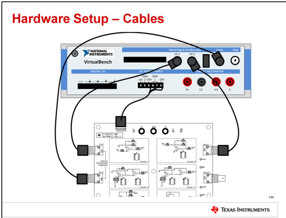
This slide gives the connection diagram between the TI Precision Labs test board and the National Instruments VirtualBench. Connect the provided power cable to the DC power supply of the Virtual Bench and power connector J4 on the test board.
