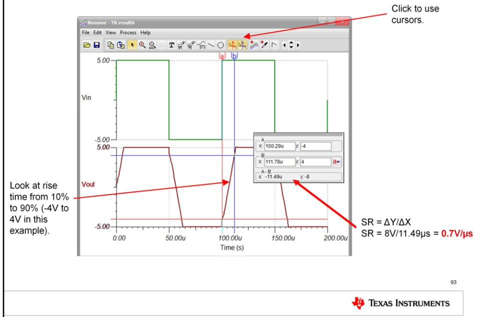
You should see a result similar to this. Vin is a square wave, as expected, but Vout must obey the slew rate limitations of the OPA277. You can see this effect in the rise time from 10% to 90% of the output, or -4V to 4V. Use the cursors to measure the time required to slew from -4V to 4V, and use the equation that slew rate = delta y over delta x to calculate the simulated slew rate of 0.7V/ $\mu$ s.
