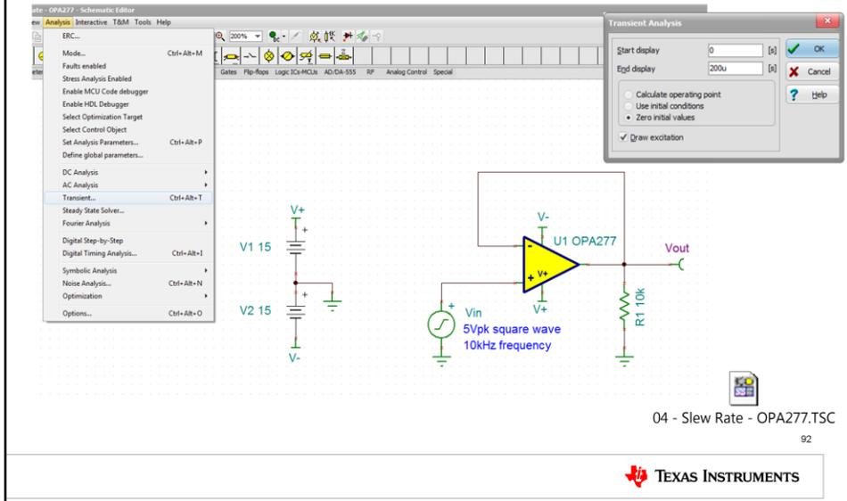
The next step is to run a SPICE simulation analysis for the transient output voltage behavior. This will allow us to see the op amp's output voltage response for a specified input signal, which in this case is a 5Vp, 10kHz square wave.
