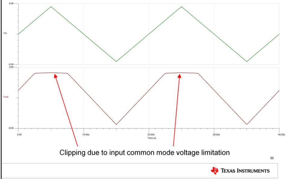
You should see a result similar to this.  $V_{in}$  is a triangle wave, as expected, but  $V_{out}$  cannot exceed +1V. This is due to the input common mode voltage limitation of the OPA735.
