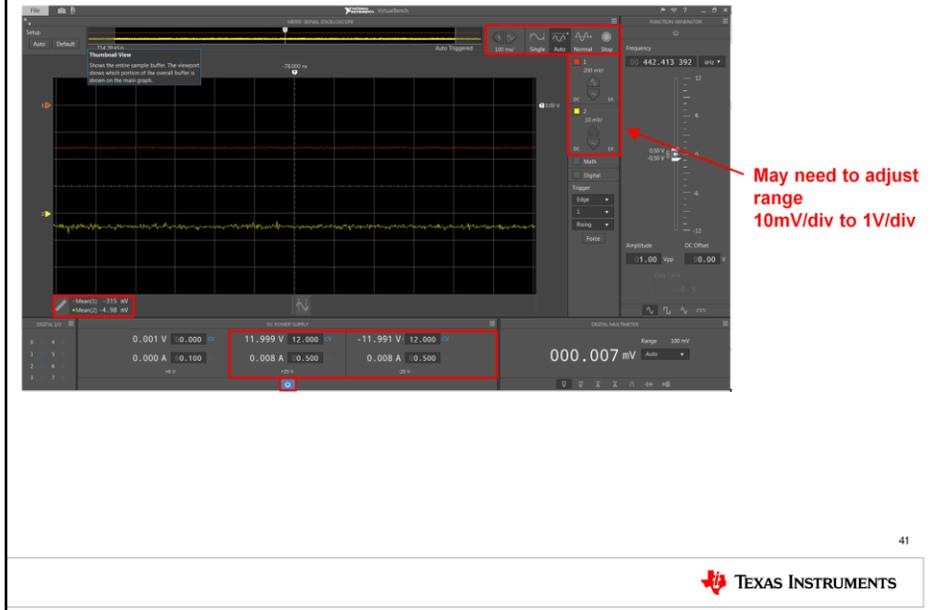
Next apply power to the National Instruments VirtualBench and connect it to your computer with a USB cable. The hardware should be detected as a virtual CD drive, and you can run the VirtualBench software directly from the drive. Once the software opens, configure the software as follows:
