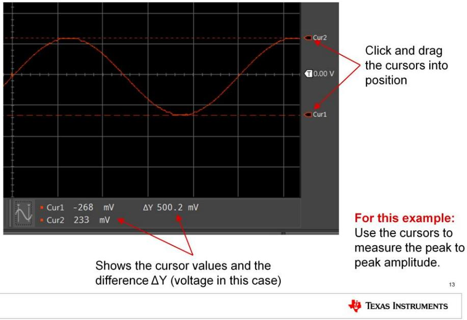
The cursors location may be adjusted to make a measurement. Click and drag the cursor indicators into position at the top and bottom of the sinusoidal waveform. The voltage level at each cursor, as well as the delta Y, in this case voltage difference, will be displayed next to the cursor icon. Use the cursors to measure the signal's peak-to-peak amplitude.
