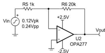
With a 0.24Vpp (0.12Vpk) input signal, is the circuit limitation caused by input common mode range or output voltage swing?
