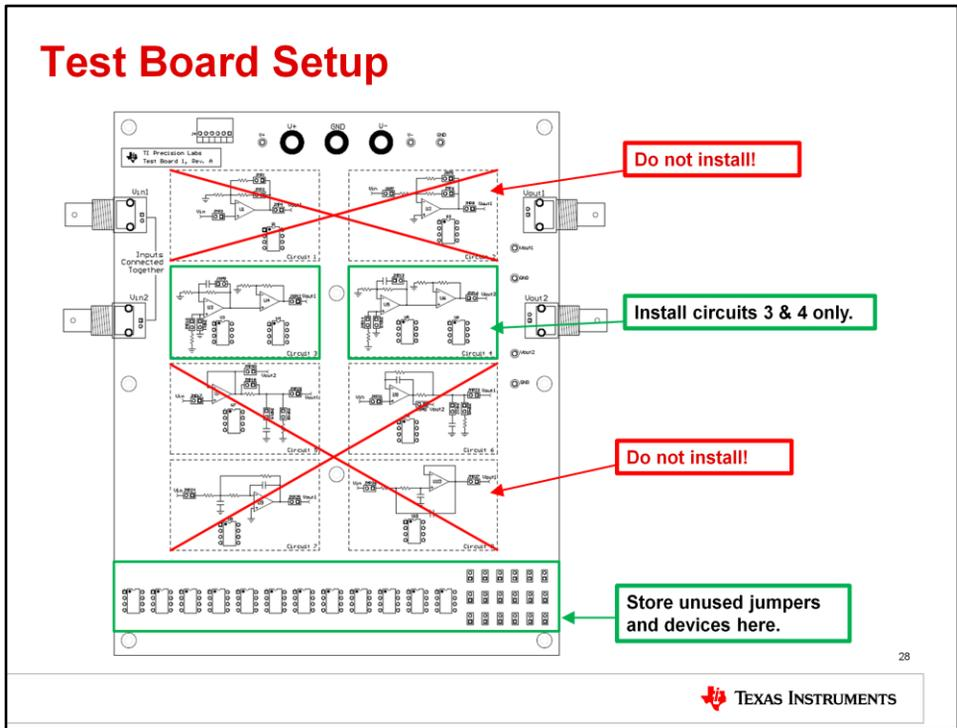
For the test board to function properly, it is important that you only install jumpers and devices in circuits 3 and 4. Do not install any jumpers or devices in any other circuits on the PCB! Remove any jumpers or devices from the unused circuits and store them in the storage area at the bottom of the test board.
