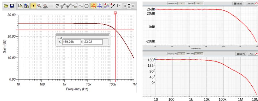
2. Compare the calculated, simulated, and measured bandwidth for the OPA171.
