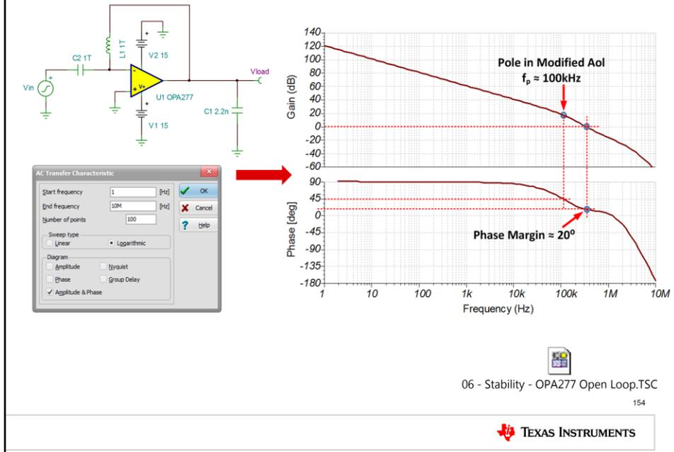
To determine the value of isolation resistor  $R_{iso}$ , we must first know the open-loop AC response of the circuit. Here we show the TINA-TI simulation schematic and AC response results, which you can verify using the embedded file.
