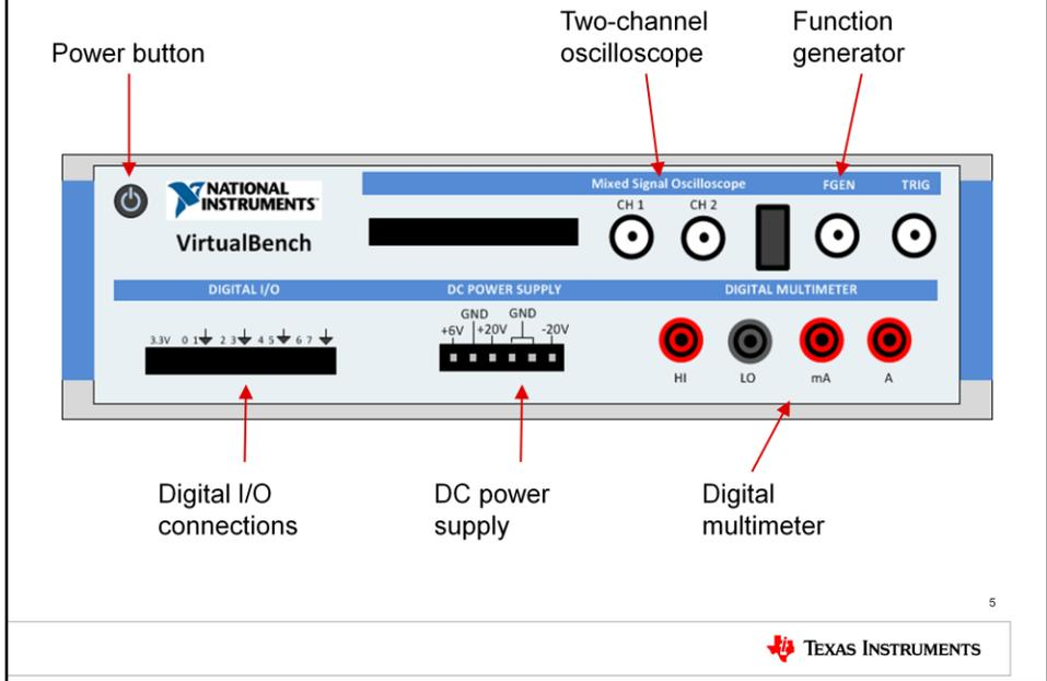
The front panel of the virtual bench is used to make connections to your system under test. You must turn on the VirtualBench by pressing the power button on the top left before using the device. Then, you can connect to the oscilloscope, function generator, digital I/O, DC power supply, and digital multimeter as required in your experiments.
