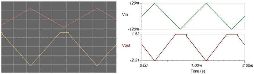
2. Use the cursors on the VirtualBench and TINA-TI™ tool to measure the voltage where Vout becomes limited (clipped). Compare this to your calculation.
