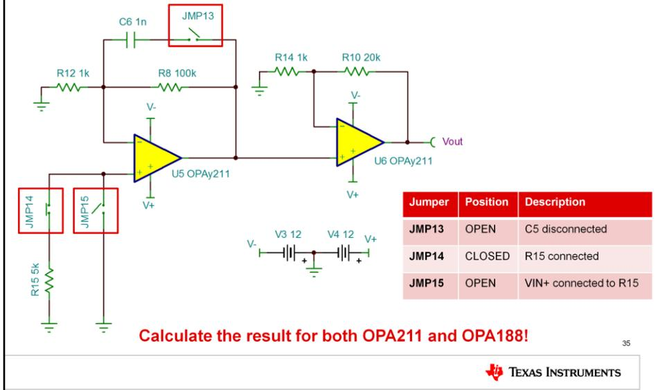
As shown in the schematic, jumper JMP15 shorting the positive input of U5 to ground is now removed. Jumper JMP14 is now installed in order to connect the positive input of U5 to a 5kΩ resistor. The  $I_B$  of U5 will now flow through this resistor, developing a DC voltage due to Ohm's law and increasing the amount of offset voltage.
