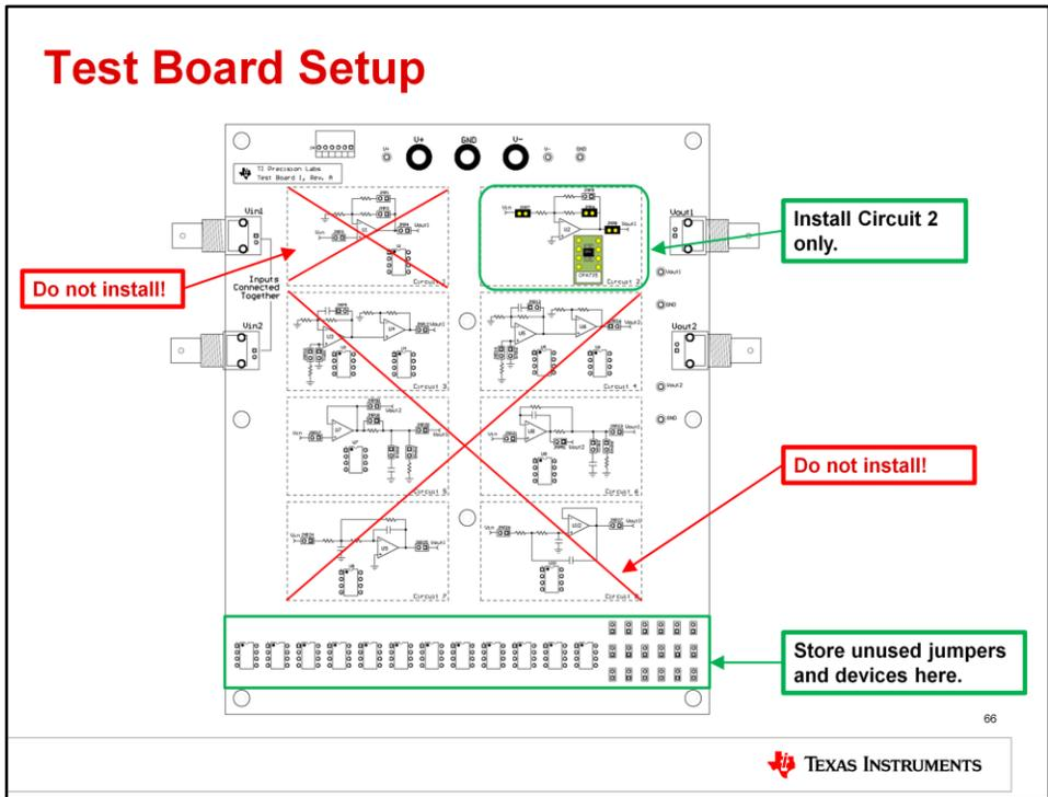
For this measurement, only circuit 2 is used. Do not install any jumpers or devices in any other circuits on the PCB! Remove any jumpers or devices from the unused circuits and store them in the storage area at the bottom of the test board.
