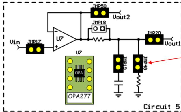
Measure transient response with JMP48 installed and removed.
