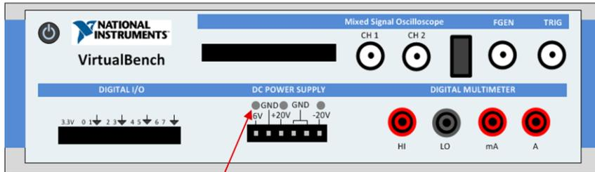
LEDs OFF = DC power supply OFF
