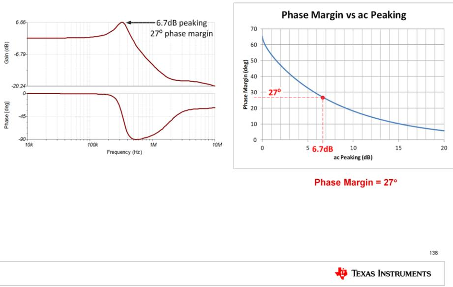
You should see a result similar to this. The 9dB of simulated AC peaking results in a phase margin of approximately 20 degrees.
