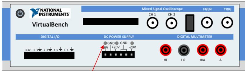
LEDs OFF = DC power supply OFF
