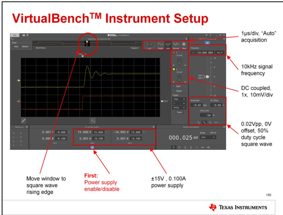
Next apply power to the National Instruments VirtualBench and connect it to your computer with a USB cable. The hardware should be detected as a virtual CD drive, and you can run the VirtualBench software directly from the drive. Once the software opens, configure the software as follows:
