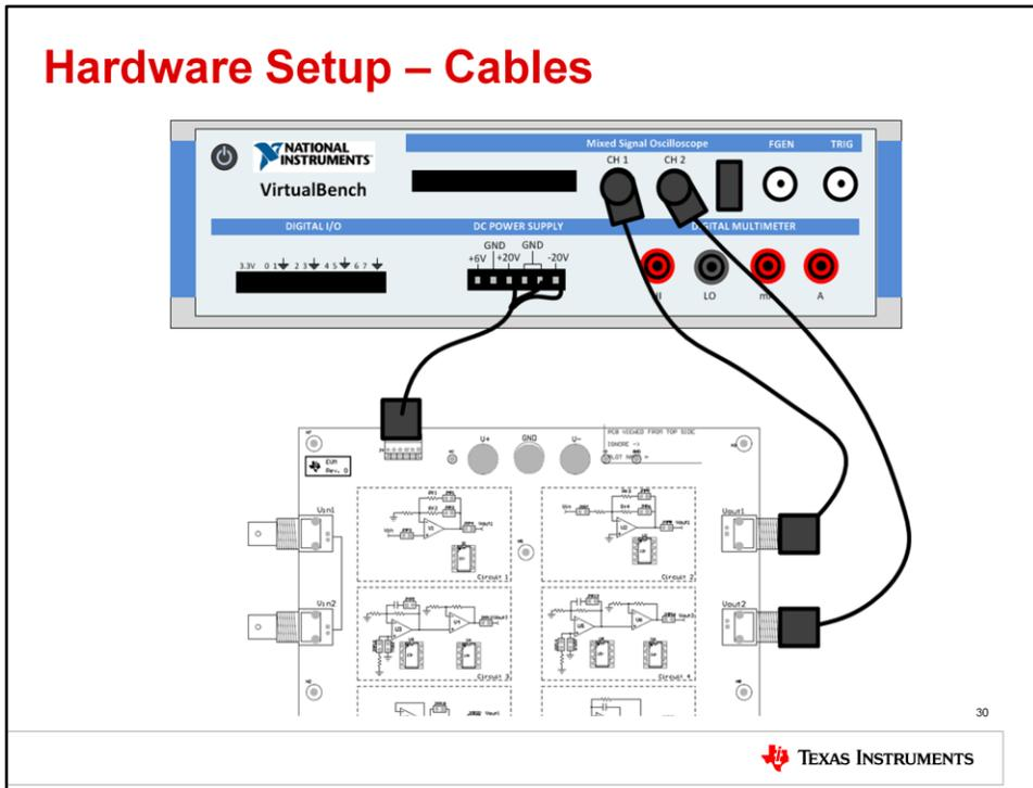
This slide gives the connection diagram between the TI Precision Labs test board and the National Instruments VirtualBench. Connect the provided power cable to the DC power supply of the Virtual Bench and power connector J4 on the test board. Connect Vout1 on the test board to VirtualBench oscilloscope channel 1, and Vout2 on the test board to Virtual Bench oscilloscope channel 2, using BNC cables.
