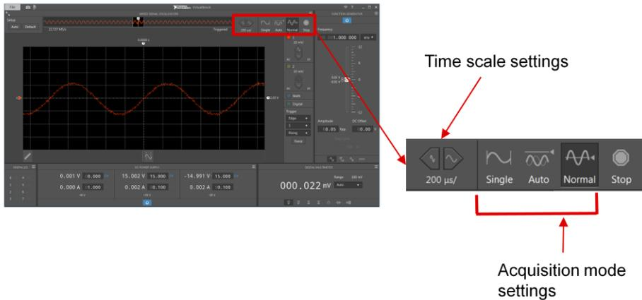
Here we set the horizontal time base on the scope as well as the triggering mode. "Auto" is untriggered roll or automatic triggering. Normal is triggered. For periodic signals it is best to use normal mode.
