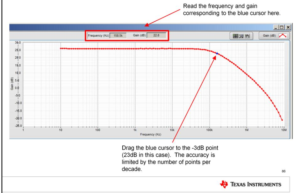
You should see a result similar to this. Enable the cursor, then drag the cursor to the -3dB point, or 23dB in this case. Take note of the frequency – in this case the result is 159kHz, although your results may vary slightly.
