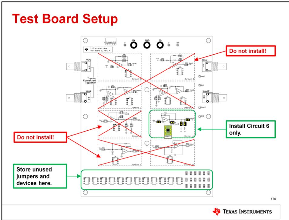
For the test board to function properly, it is important that you only install jumpers and devices in circuit 6! Do not install any jumpers or devices in any other circuits on the PCB! Remove any jumpers or devices from the unused circuits and store them in the storage area at the bottom of the test board.
