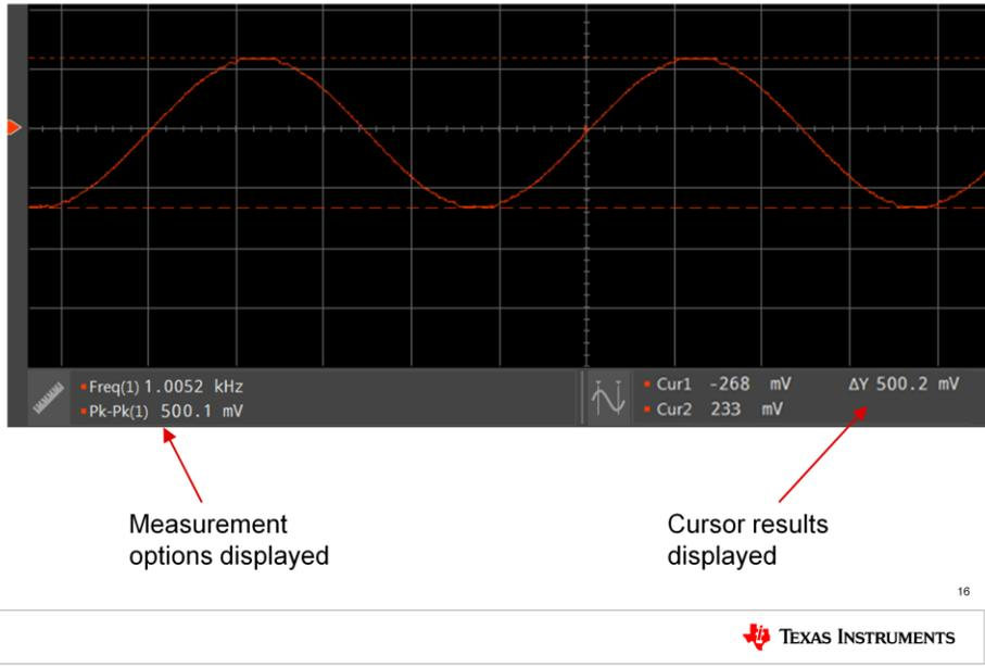
The measurement results are displayed next to the ruler icon. You should read a result of 1kHz, 500mVpp – the same as the function generator. The amplitude should be the same as the delta Y measurement from the cursor.
