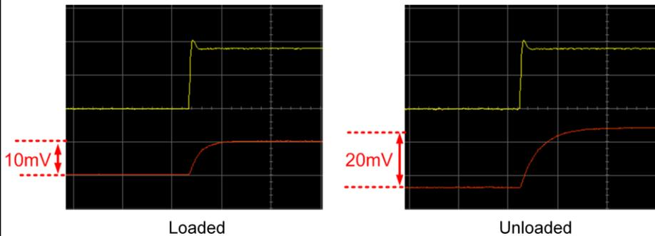
**$R_{ISO}$  can cause significant attenuation when under load!**
