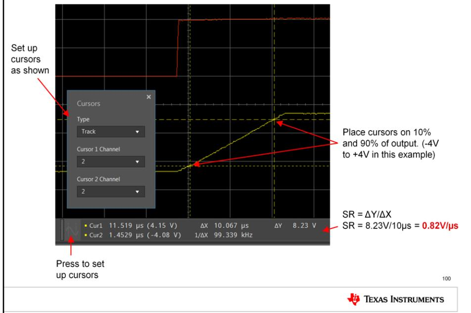
Let's now determine the measured slew rate. Enable cursors, set them up as shown, then place the cursors on 10% and 90% of the output signal. Take note of the time and voltage difference, and then calculate the slew rate using the equation given. In this example, a slew rate of  $0.82\text{V}/\mu\text{s}$  was measured. You may have different results in your experiment.
