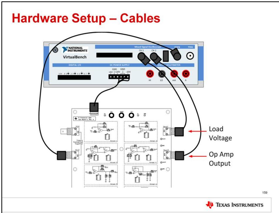
This slide gives the new connection diagram between the TI Precision Labs test board and the National Instruments VirtualBench. Connect the provided power cable to the DC power supply of the Virtual Bench and power connector J4 on the test board.
