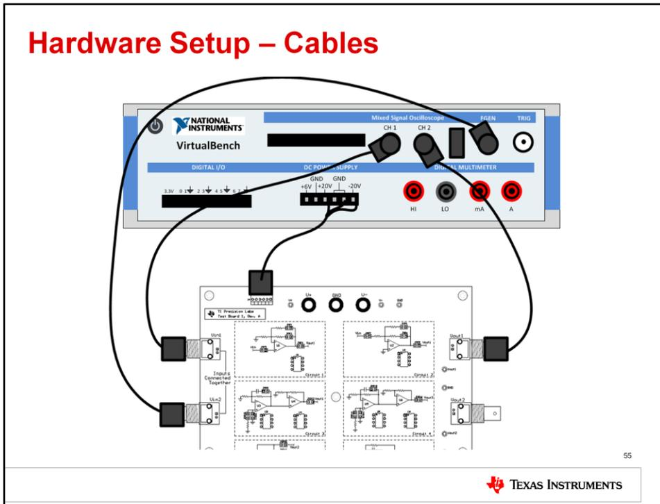
This slide gives the connection diagram between the TI Precision Labs test board and the National Instruments VirtualBench. Connect the provided power cable to the DC power supply of the Virtual Bench and power connector J4 on the test board. Connect Vin2 on the test board to VirtualBench channel FGEN, or function generator. Then connect Vin1 on the test board to VirtualBench oscilloscope channel 1, and Vout1 on the test board to VirtualBench oscilloscope channel 2.
