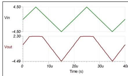
2. Use the cursors on the VirtualBench and TINA-TI™ tool to measure the voltage where Vout becomes limited (clipped). Compare this to your calculation.
