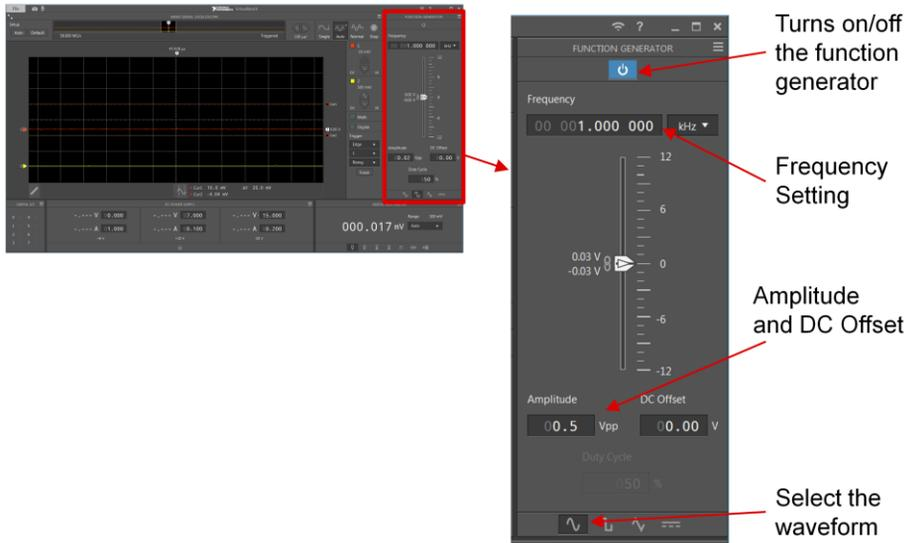
The image shows a screenshot of a function generator interface. On the left, a smaller window displays a waveform on a grid. On the right, a larger window titled 'FUNCTION GENERATOR' shows the configuration settings. Red arrows point from text labels to specific controls in the interface:
