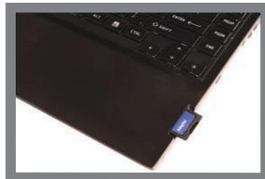
**8** To prepare your workstation for software development, power off the kit, remove the microSD card and insert it into your Ubuntu Linux workstation (adapter may be required). If your workstation does not include an SD slot, USB SD card adapters are readily available. Follow the instructions to the right
