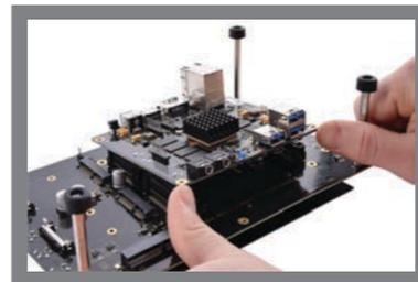
If necessary to unplug the Processor Module, it is recommended to do so by pushing up from the corners as shown in the picture to minimize risk of damage.
