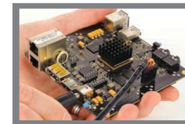
**5** Connect the supplied power cable to the processor board as shown (for simplicity only the processor board is shown). Connect the **12-volt power supply** cable to an AC power source.
