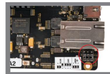
**4** Confirm the jumpers J3, J4, J6 are jumpered across positions 2 and 3 (closest to edge of board).
