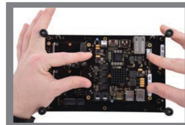
Similarly, it is recommended to plug back in the Processor Module by pressing down on the sides of the Processor Module as shown in the picture to minimize risk of damage.
