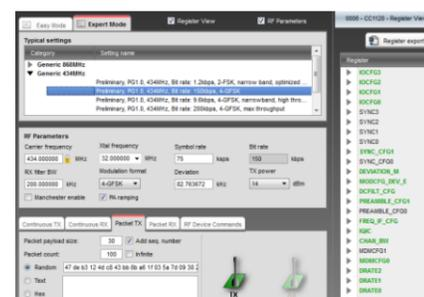
You can now configure the radio, run performance tests, export register settings and run link tests with another CC1120 on a SmartRF TrxEB connected to the PC.
