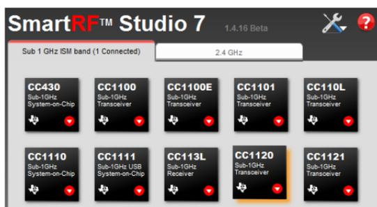
After installing the tool, connect the EB to the PC using the USB cable and start SmartRF Studio. Select the "Sub 1 GHz" tab and double click the highlighted CC1120 device icon.
