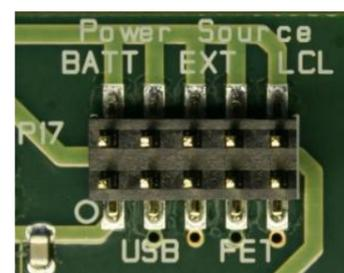
Depending on the power source, make sure you connect jumpers to the appropriate pins on the "Power Source" header. For instance, if you use batteries, use a jumper to short-circuit pin 1 and 2 on the header. See back side of board for explanation of the jumpers.
