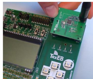
Insert a CC1120EM board into the TrxEB as shown above. Connect the antenna firmly to the SMA connector on the EM.
