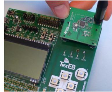
Insert a CC112xEM board into the TrxEB as shown above. Connect the antenna to the SMA connector on the EM.
