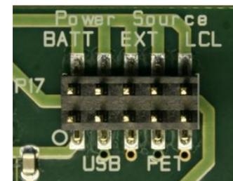
Depending on the power source, make sure you connect jumpers to the appropriate pins on the “Power Source” header. For instance, if you use batteries, use a jumper to short-circuit pin 1 and 2 on the header. The last jumper in the row (pin 9-10) should always be mounted, unless the MSP430 FET is used as the power source.
