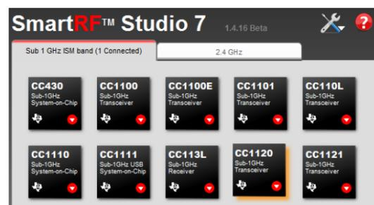
After installing the tool, connect the EB to the PC using the USB cable and start SmartRF Studio. Select the "Sub 1 GHz" tab and double click the highlighted CC1120 or CC1121 device icon.
