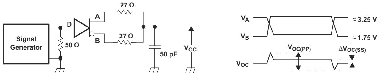
**图 7-5. Driver  $V_{OC}$  Test Circuit and Waveforms**
