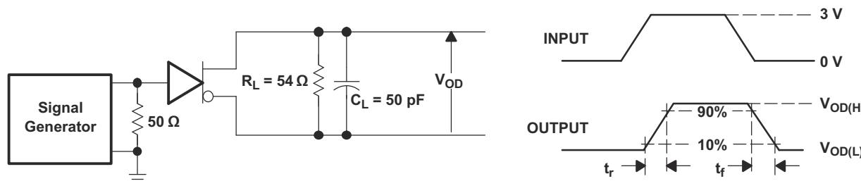
図 7-3. Driver Switching Test Circuit and Rise/Fall Time Measurement
