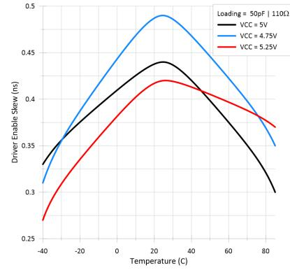
**图 6-5. Driver Enable Skew vs Free-Air Temperature**
