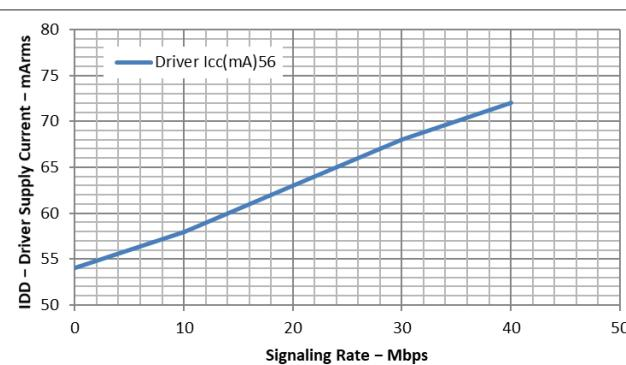
**图 6-2. Driver Supply Current vs Signaling Rate**
