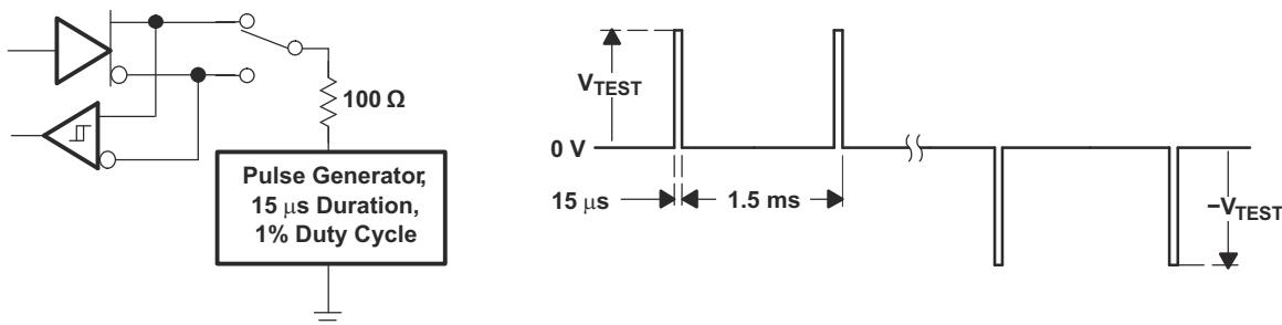
**图 7-15. Test Circuit and Waveforms, Transient Overvoltage Test**
