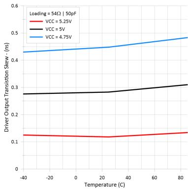
**图 6-3. Driver Output Transition Skew vs Free-Air Temperature**
