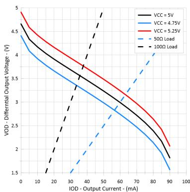
**图 6-1. Differential Output Voltage vs Load Current**
