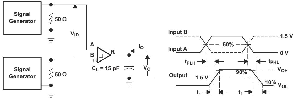
図 7-10. Receiver Switching Test Circuit and Waveforms
