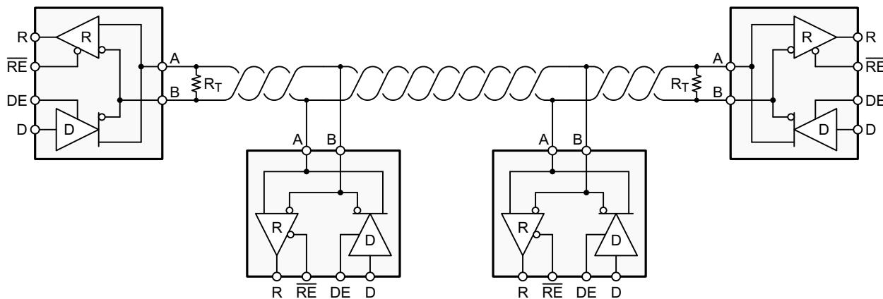
図 8-2. Typical RS-485 Network With Half-Duplex Transceivers
