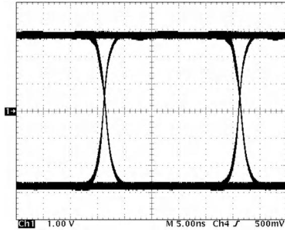
**图 8-6. Differential Output of SN65HVD1176 Operation at 40 Mbps**
