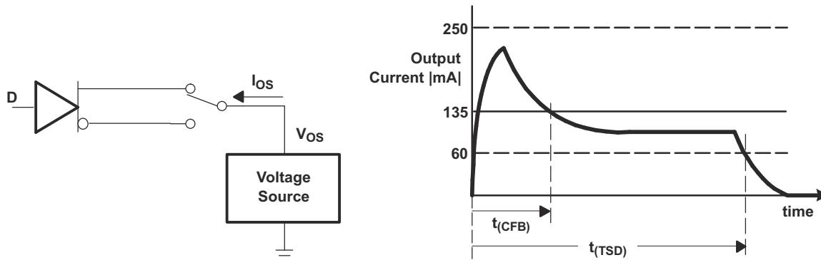
図 7-8. Driver Short-Circuit Test Circuit and Waveforms (Short Circuit applied at Time  $t = 0$ )
