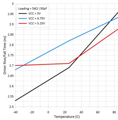
**图 6-4. Driver Rise, Fall Time vs Free-Air Temperature**
