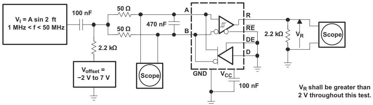
図 7-11. Receiver Common-Mode Rejection Test Circuit
