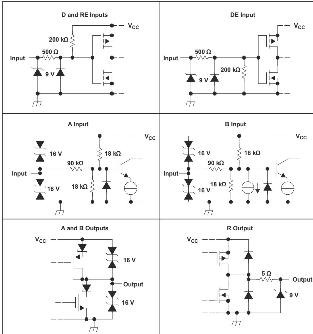
**図 7-2. Equivalent Input and Output Schematic Diagrams**
