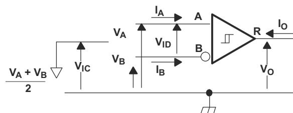
図 7-9. Receiver DC Parameter Definitions
