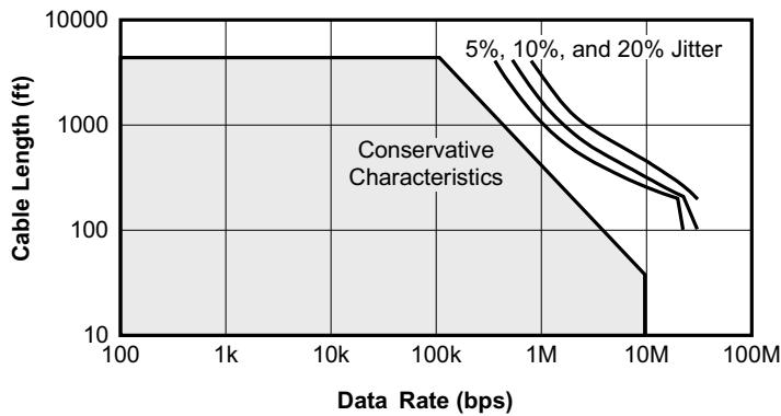
**図 8-4. Cable Length vs Data Rate Characteristic**
