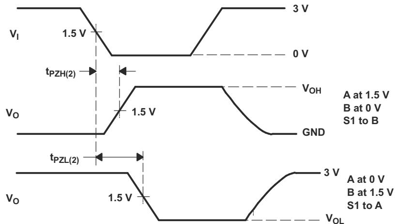
**FIGURE 7-12. Receiver Enable Time From Standby (Driver Disabled)**
