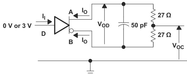
図 7-1. Driver Test Circuit,  $V_{OD}$  and  $V_{OC}$  Without Common-Mode Loading
