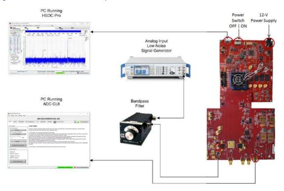
Figure 3. EVM Test Setup
