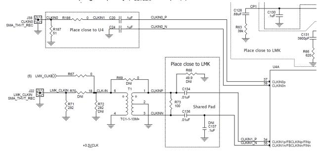
Figure 10. External LMKCLK Configuration
