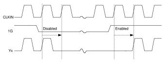
Figure 2. Synchronous Output Enable
