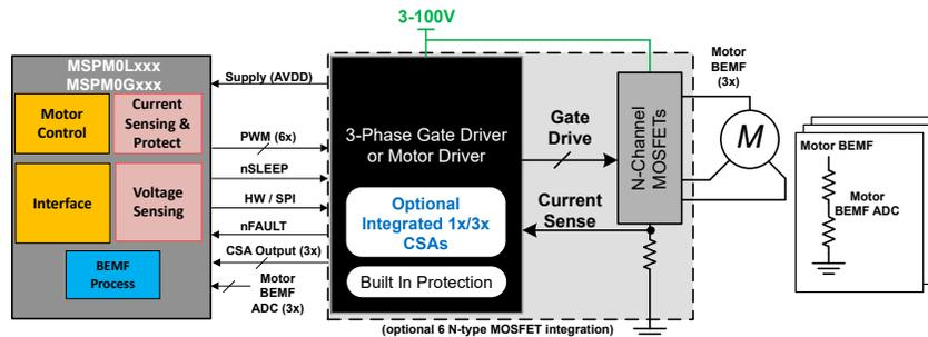
Figure 4. MSPM0 Block Diagram for Sensorless Trapezoidal Control
