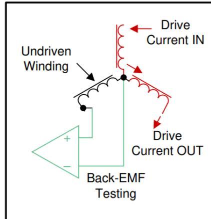
**Figure 2. BEMF Detection using Comparator on Undriven Winding**
