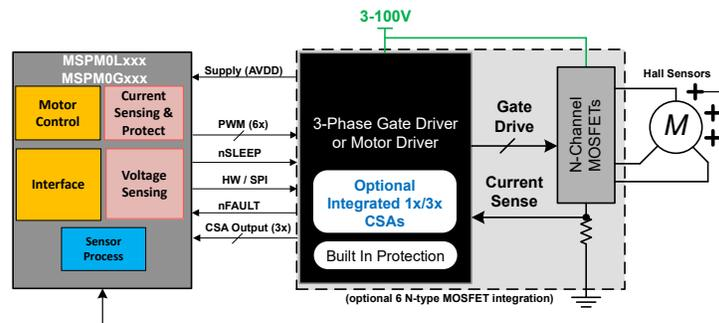
Figure 3. MSPM0 Block Diagram for Hall-Sensored Trapezoidal Control
