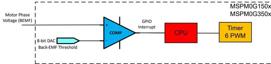
**Figure 7. MSPM0 COMP Block Diagram for BEMF Detection**
