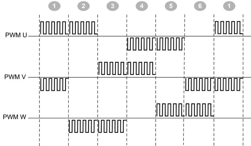
Figure 5. PWM Sequence for 120° 6-Step TRAP
