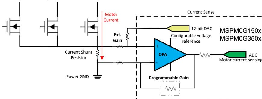
Figure 6. MSPM0Gx OPA Block Diagram for Current Sensing
