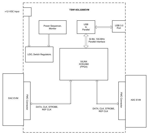
Figure 2. TSW14DL3200EVM Block Diagram
