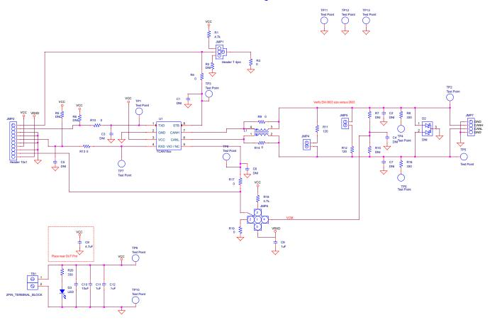
Figure 3. TCAN1042DEVM Schematic Evaluation Board Used to Perform the SEL
