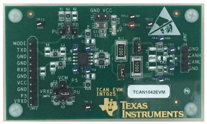
Figure 2. SN55HVD233-SEP Mounted on TCAN1042DEVM
