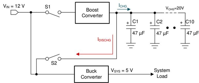
**Figure 1. Simplified Application Circuit for the Hold-up Function**
