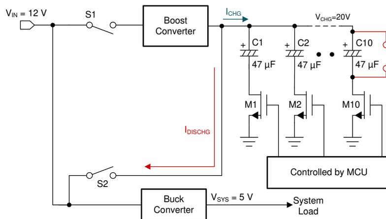
**Figure 2. Simplified Schematic for Better Reliability Using CSD16327Q3**
