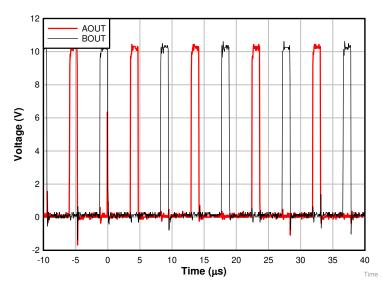
Figure 14. Worst-Case Negative Deviation From the Nominal Pulse Width on A-OUT
