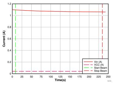
Figure 9. V<sub>cc</sub> and V<sub>IN</sub> Current vs Time for SEB Run #2 at T = 125°C and 74.1 MeV·cm<sup>2</sup>/mg
