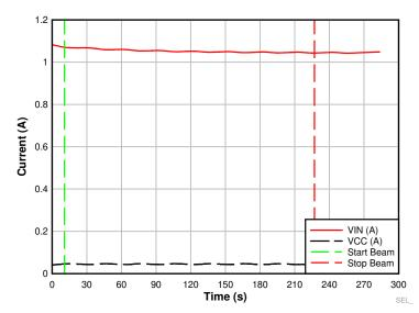
Figure 8.  $V_{cc}$  and  $V_{IN}$  Current vs Time for SEL Run #1 at T = 125°C and 74.1 MeV·cm<sup>2</sup>/mg
