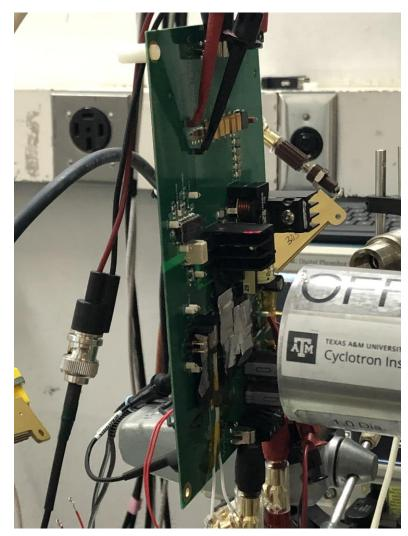
Figure 5. Photograph of the UC1825B-SP Mounted on the UC1825BEVM-CVAL EVM in Front of the Heavy-ion Beam Exit Port at the TAMU Accelerator Facility
