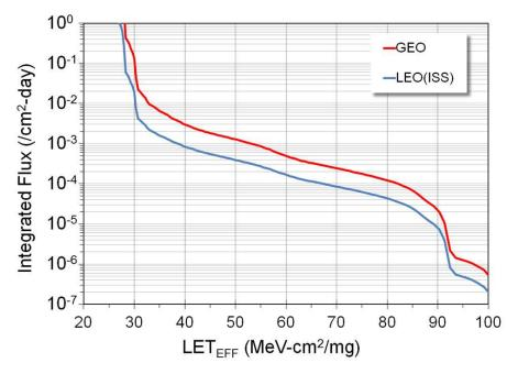
LEO(ISS) (blue) and a GEO (red) environment as calculated by CREME96, assuming worst-week and 100 mils (2.54 mm) of aluminum shielding.
