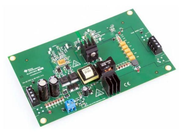
Figure 2. UC1825B-SP EVM Top View
