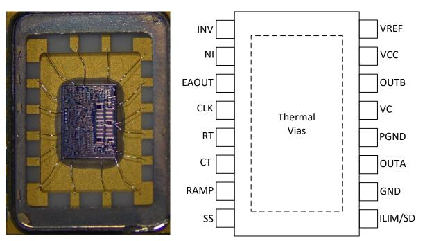
The package lid was removed to reveal the die face for all heavy-ion testing.
