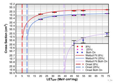
Figure 10. A-OUT Cross Section vs LET for the 10-A Load on the UC1825B-SP
