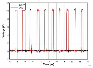
Figure 13. Worst-Case Positive Deviation from the Nominal Pulse Width on A-OUT
