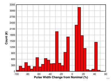
Figure 12. Histogram of all Saved Normalized Upsets in the A-OUT PWM Output ≥ |6%|
