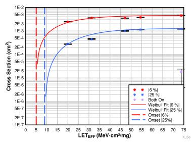
Figure 11. A-OUT Cross Section vs LET for the 1-A Load on the UC1825B-SP
