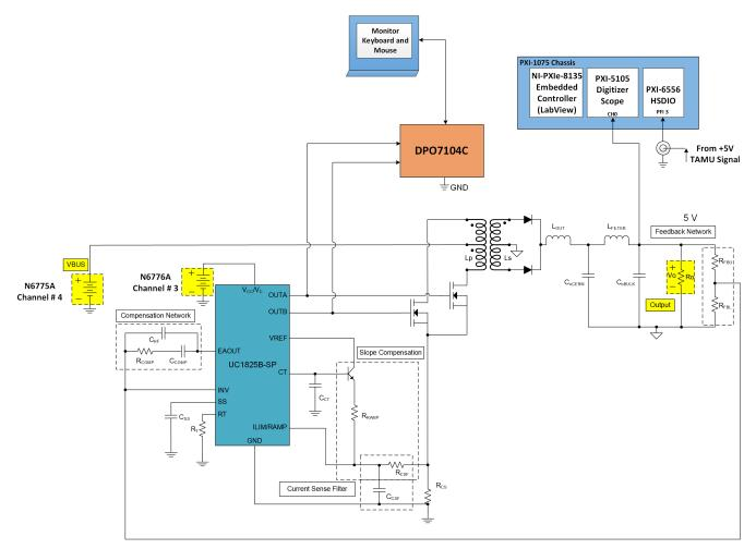
Figure 7. Block Diagram of the Test Setup Used for UC1825B-SP SEE Characterization
