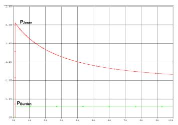
Figure 3-4. Power Dissipation in Zener and Burden Resistor During Miswiring Faults
