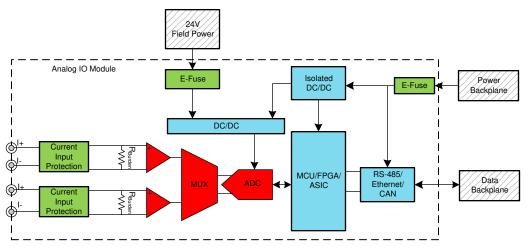
Figure 1-1. Current input protection in Analog Input modules
