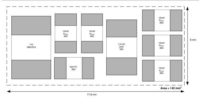
Figure 3-5. PCB Size with Multiple Burden Resistors
