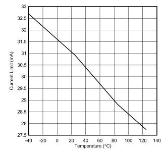
Figure 4-2. Current Limit with TPS26610
