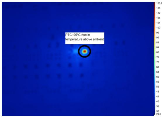
Figure 3-7. Temperature rise with Discrete Circuit
