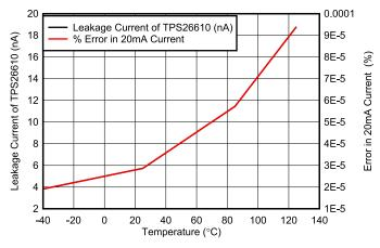
Figure 4-3. Leakage Current of TPS26610
