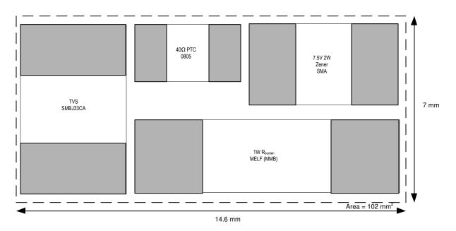
Figure 3-6. PCB Size with MELF Resistor
