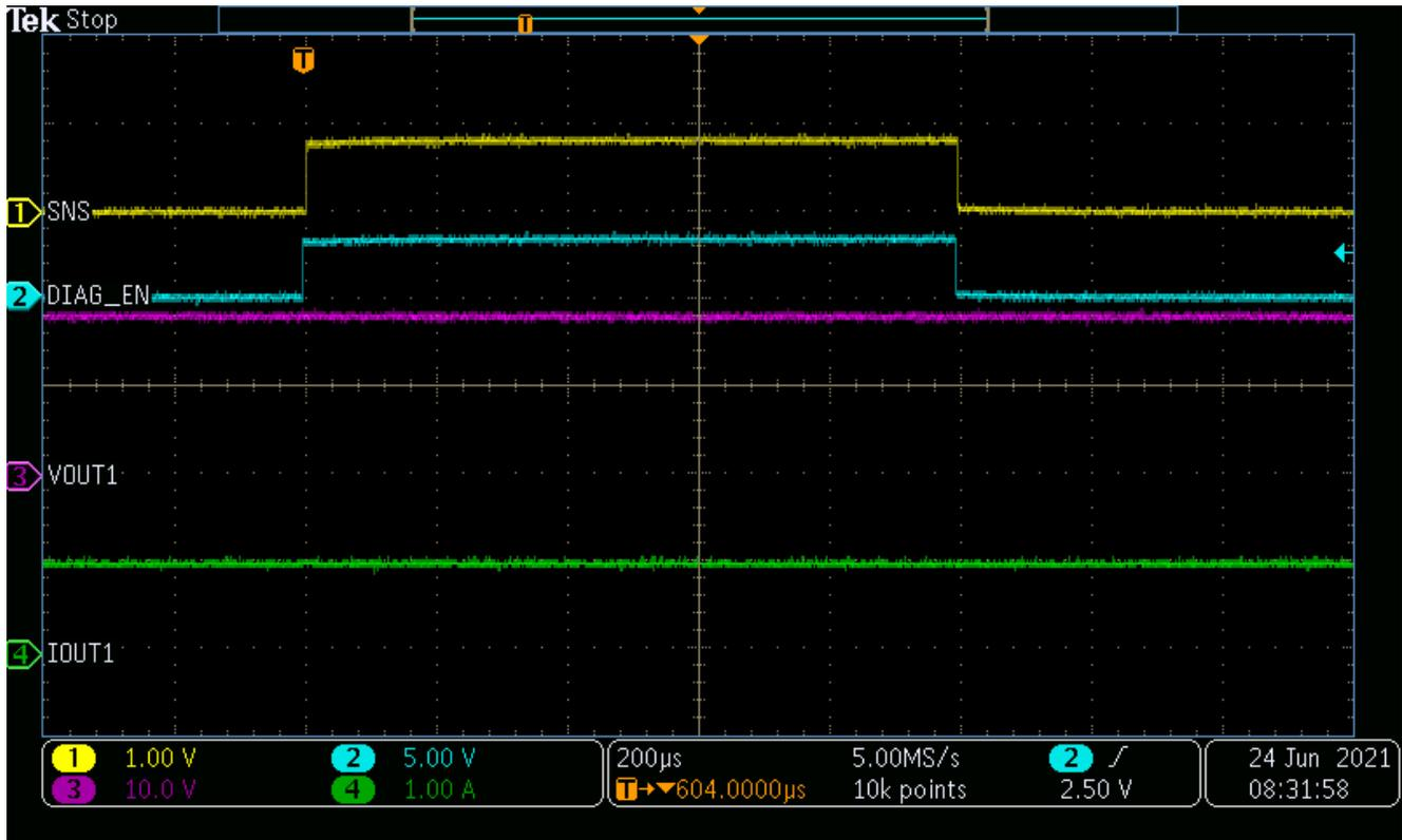
**Figure 2-3. Current Sense with DIAG\_EN Toggling**
