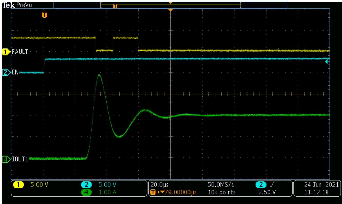
Figure 3-2. Current Limit - Permanent Short 2A
