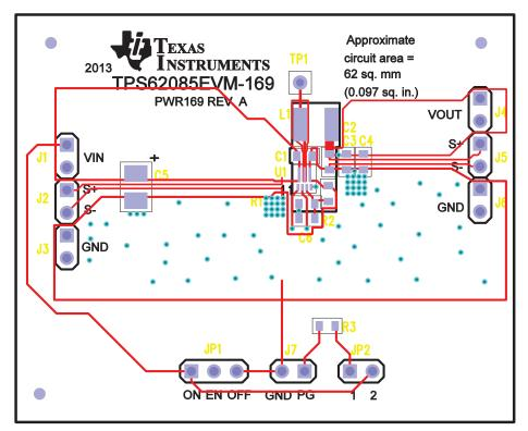
Figure 4. Assembly Layer
