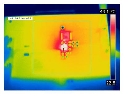
Figure 2. Thermal Performance ( $V_{IN} = 6 \text{ V}$ , Load = 3 A)
