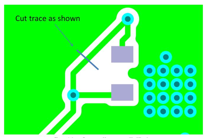
Figure 1. Loop Response Measurement Modification
