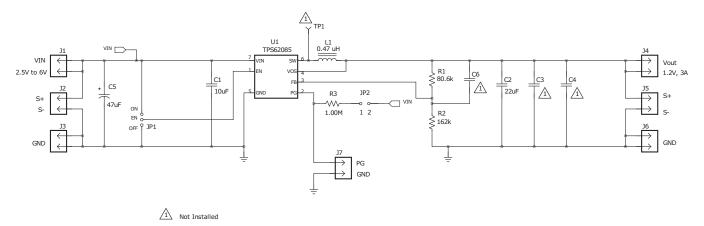
Figure 8. TPS62085EVM-169 Schematic
