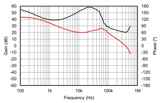
Figure 3. Loop Response Measurement (V<sub>IN</sub> = 3.6 V, Load = 3 A)
