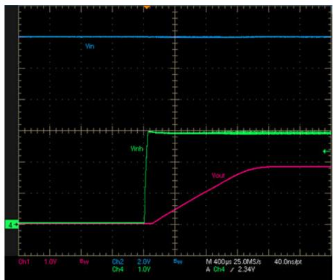
Figure 6-3. INH Start-Up Waveform
