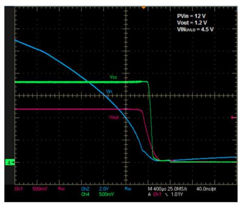
Figure 6-2. UVLO Shutdown Waveform
