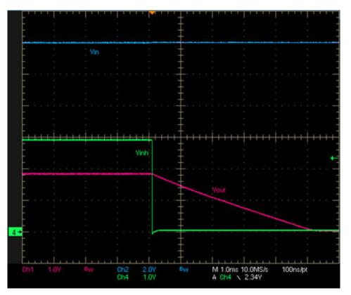
Figure 6-4. INH Shutdown Waveform
