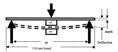
Figure 23. PCB Bend Test for the 24L CSP as Mounted to 1.6mm thick FR-4 Board
