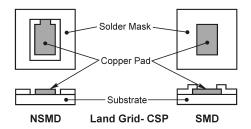
Figure 5. Comparison of NSMD and SMD pads (Laminate CSP)
