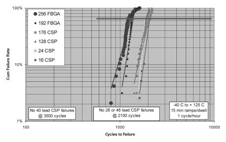
Figure 21. Solder Joint Reliability Weibul Plot
