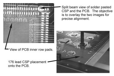
Figure 17. Component Placement.
