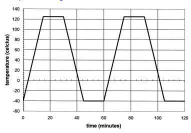
Figure 20. Temperature Cycle Test Condition Profile
