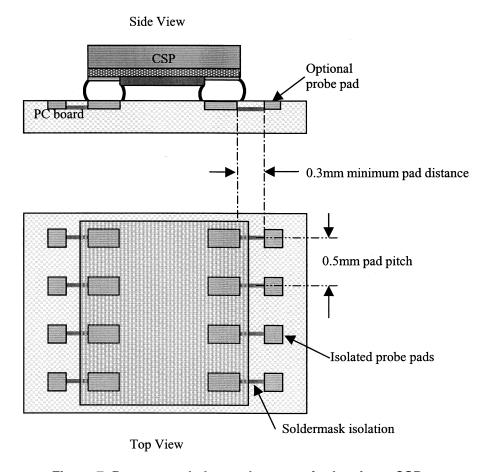
Figure 7. Recommended part placement for Laminate CSP
