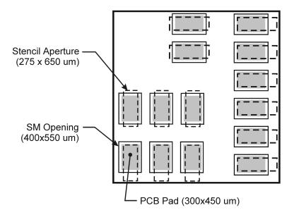
Figure 6. Stencil Design Guidlines
