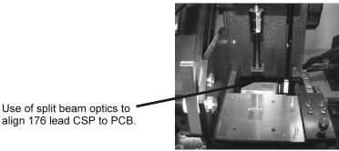
Figure 16. Component Alignment.
