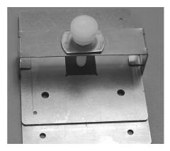
Figure 14. Rework Fixture and Rework Stencil for 176L CSP
