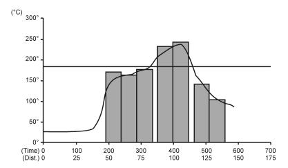
Figure 8. Typical Reflow Profile for Laminate CSP
