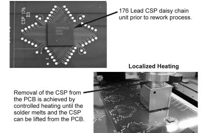
Figure 10. Removing Component from the PCB.
