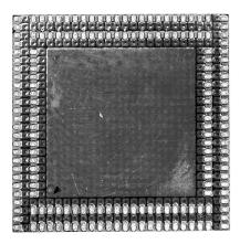
Figure 15. Solder Paste Deposition on 176L CSP
