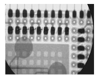
Figure 19. X-ray Inspection of 176L CSP
