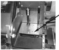
176 lead CSP on vacuum nozzle after removal from solder paste fixture.
