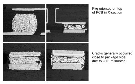
Figure 22. Laminate CSP Solder Joint Failure Mode in TMCL
