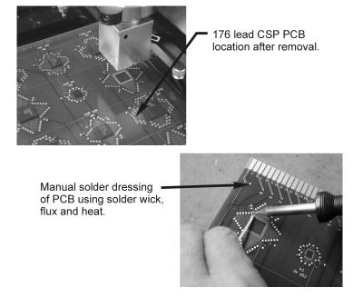
Figure 11. Dressing PCB Footprint for New CSP
