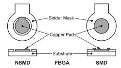
Figure 4. Comparison of NSMD and SMD pads (FBGA)
