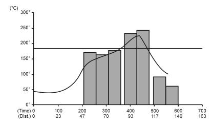
Figure 9. Typical Reflow Profile for FBGA
