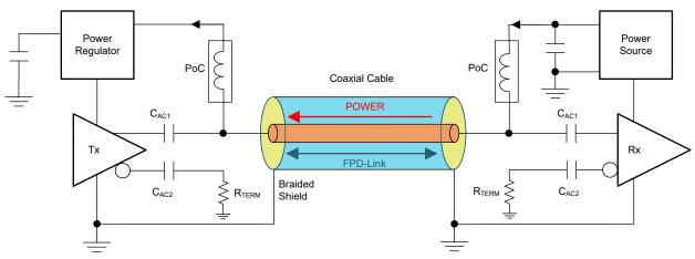
Figure 2-1. Concept for Power Over Coax
