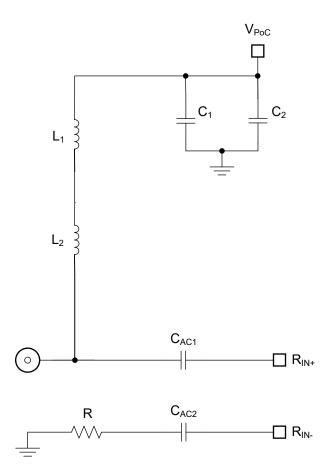
Figure 5-4. Murata PoC Network 3 Schematic
