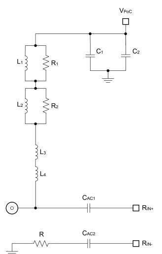
Figure 5-14. Coilcraft PoC Network 2 Schematic
