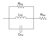
Figure 2-8. Real-World Ferrite Bead
