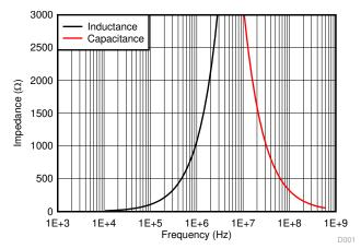
Figure 2-3. Real-world Inductor Impedance - 100 µH Inductor
