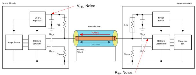
Figure 4-1. PoC Noise Measurement Nodes
