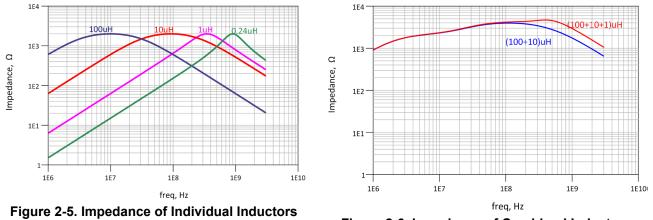
Figure 2-6. Impedance of Combined Inductors
