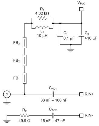
Figure 5-1. PoC Network from FPD-Link III Data Sheet Schematic
