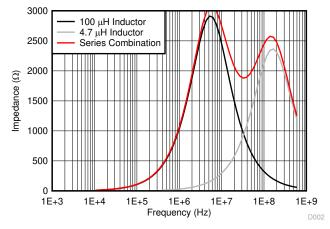
Figure 2-4. Impedance of Series Inductors
