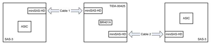
Figure 7. SAS-3 System Test Setup
