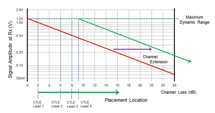
Figure 5. Illustration of Channel Extension and DS125BR820 Placement
