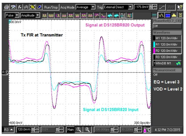
Figure 3. Transmitted and Recovered SAS-3 Waveforms
