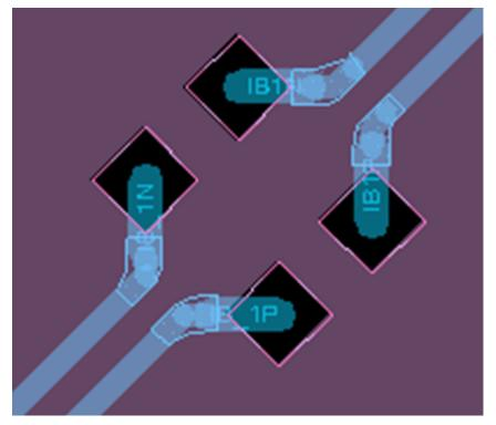
Figure 14. AC Coupling Capacitor Footprint Relief
