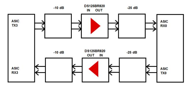
Figure 10. 12 Gbps SAS-3 Testing with System ASIC
