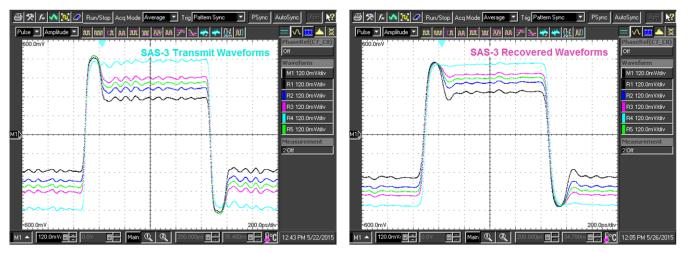
Figure 6. Waveforms at the SAS-3 Tx and After the Linear Equalizer
