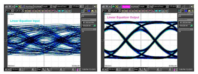
Figure 4. Waveforms Before and After a Linear Equalizer
