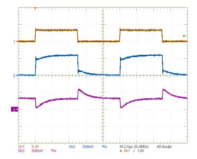
The following scope plot shows the waveforms at positive and negative inputs of the receiver (channels 2 and 3, respectively) and the differential signal resulting from them (channel M1).
