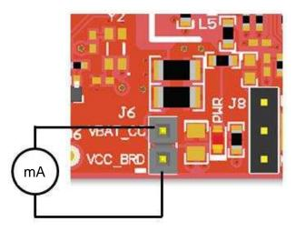
**Figure 9. Low Current Measurement**
