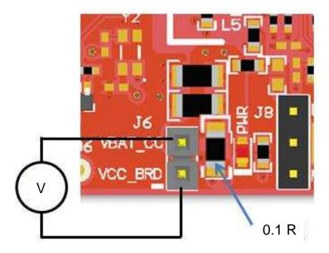
Figure 10. Active Current Measurement
