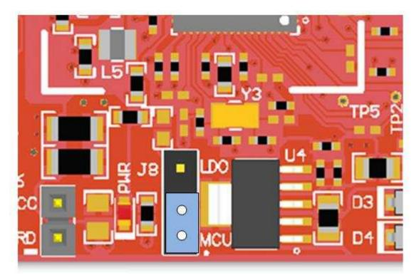
Figure 5. 3.3-V Power From MCU LaunchPad Kit
