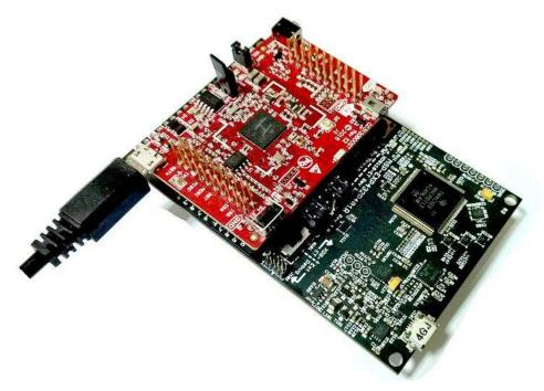
Figure 16. CC3120BP Connected to MSP432™ LaunchPad
