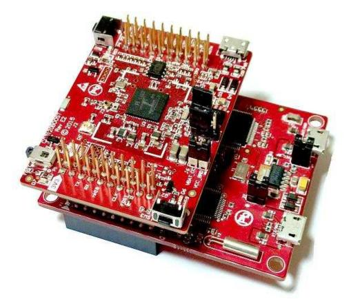
Figure 15. CC3120BOOST Connected to the CC31XXEMUBOOST Board
