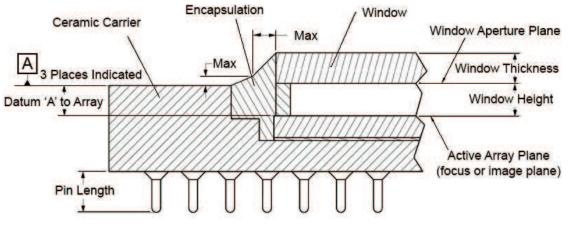
Figure 4. Series-450 DMD Cross Section View Features
