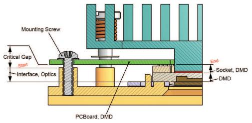
Figure 20. PC Board Gap Analysis Schematic
