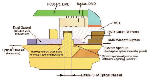
Figure 14. System Aperture and Gasket
