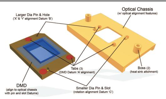
Figure 12. Optical Interface (Alignment) Features
