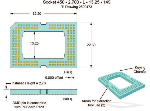
Figure 27. Low Insertion Force Style s450 Socket
