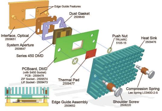
Figure 18. DMD Mounting Concept – Edge Guide
