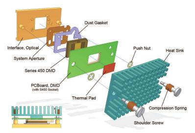
Figure 11. Basic DMD Mounting Concept
