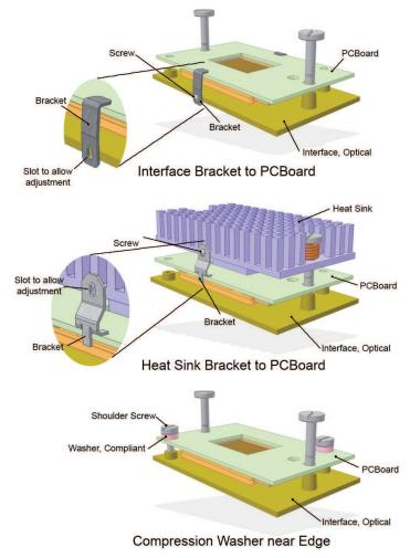
Figure 16. DMD PCBoard Direct Control Mounting Techniques
