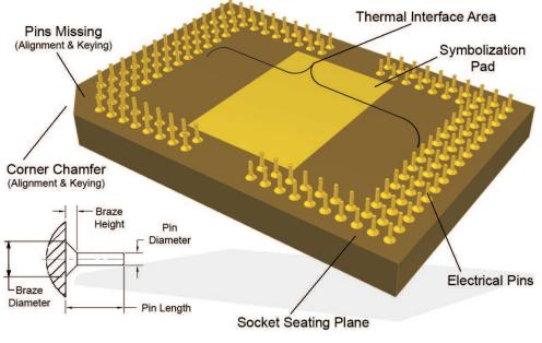
Figure 8. Electrical and Thermal Interface
