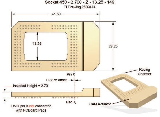
Figure 26. Zero Insertion Force Style Series-450 Socket
