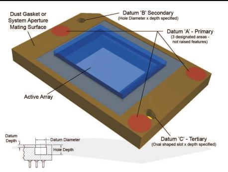
Figure 3. Series-450 DMD Datum Features and Gasket Aperture Surface
