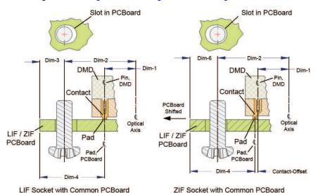
Figure 23. Contact Offset (Common PCBoard)
