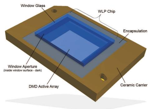
Figure 1. Series-450 DMD Features – Window Side
