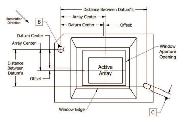
Figure 6. Active Array Location
