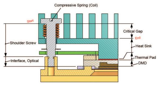
Figure 19. Heat Sink Mounting Tolerance Analysis Schematic
