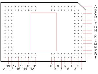
Figure 7. Pin Numbering Scheme
