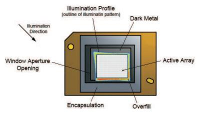
Figure 5. Optical Illumination Overfill
