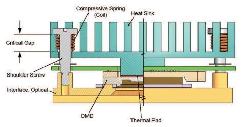
Figure 13. Heat Sink Mounting Critical Gap
