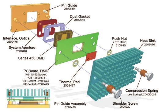
Figure 21. DMD Mounting Concept – Pin Guide
