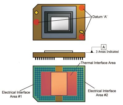
Figure 10. DMD Mechanical Loads
