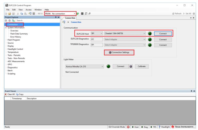
Figure 5. Connecting to the DLPC230-Q1 Using the DLPC230-Q1 Automotive Control Program
