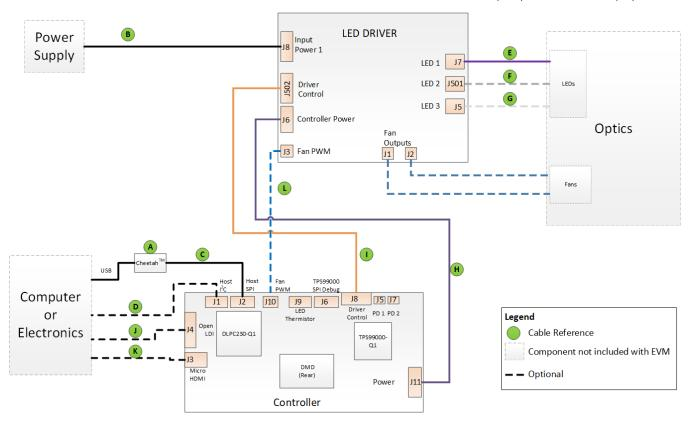
Figure 4. EVM Cable Connections
