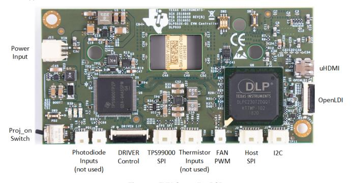
Figure 1. EVM Controller PCB
