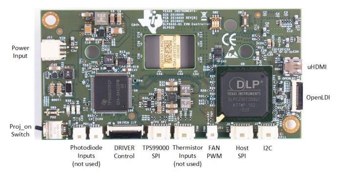
Figure 2. EVM Controller PCB
