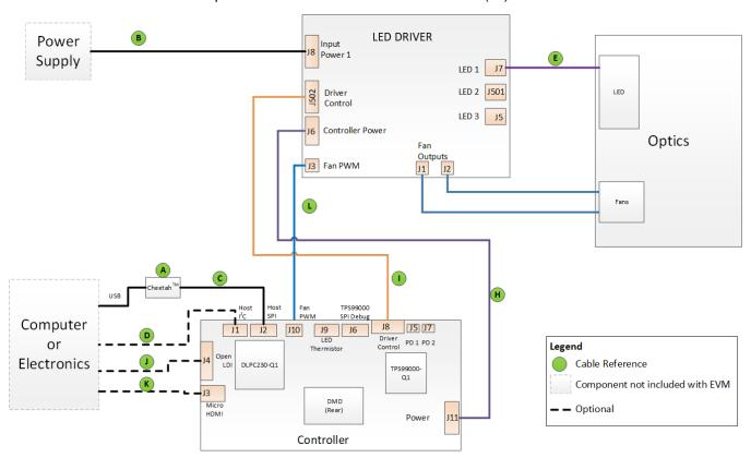
Figure 5. EVM Cable Connections
