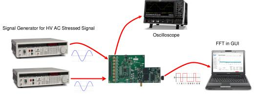
Signal Generator for AC Test Signal
