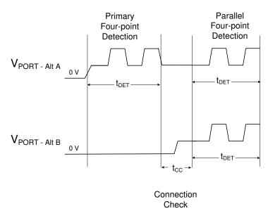
図 42. 4-Pair Port, Detection and Connection Check Waveforms with a Dual Signature Load
