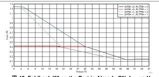
図 40. Foldback When the Port is Already ON: I<sub>LIM</sub> vs V<sub>drain</sub>
