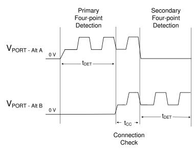
図 41. 4-Pair Port, Detection and Connection Check Waveforms with a Single Signature Load
