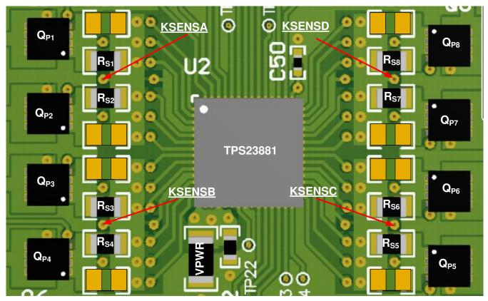
Note: PCB layout includes footprints for optional parallel  $R_{\text{SENSE}}$  resistors
