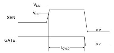
図 32. Overcurrent Fault Timing
