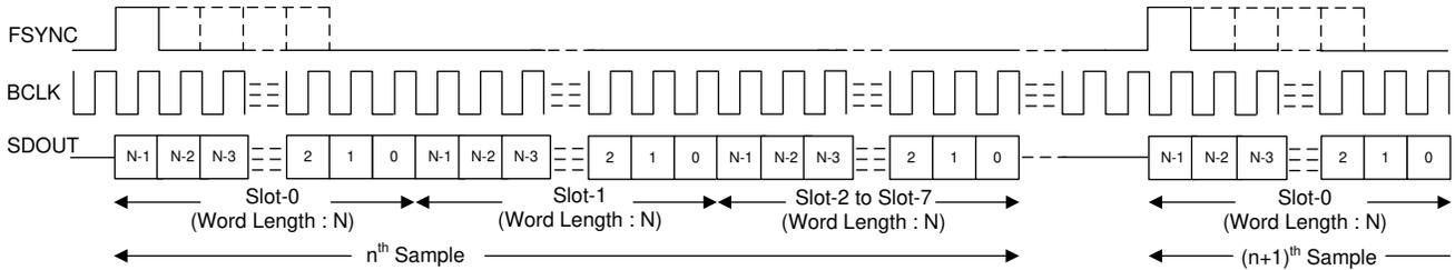
图 8-4. TDM Mode Protocol Timing (TX\_OFFSET = 0 and BCLK\_POL = 1)
