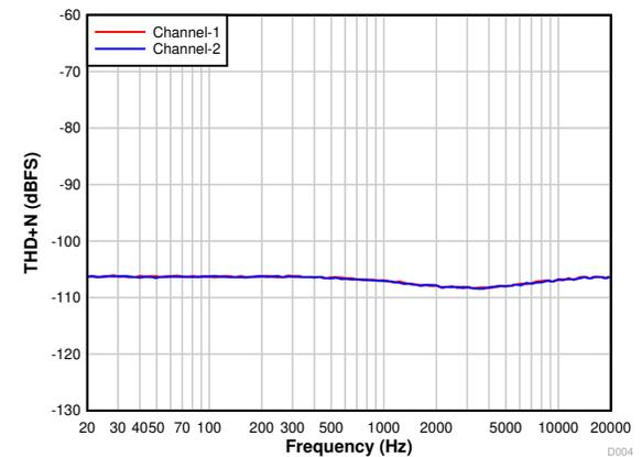
7-7. THD+N vs Input Frequency With a  $-60\text{-dBr}$  Input
