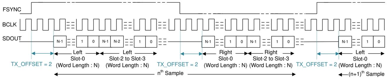
图 8-10. LJ Protocol Timing (TX\_OFFSET = 2)
