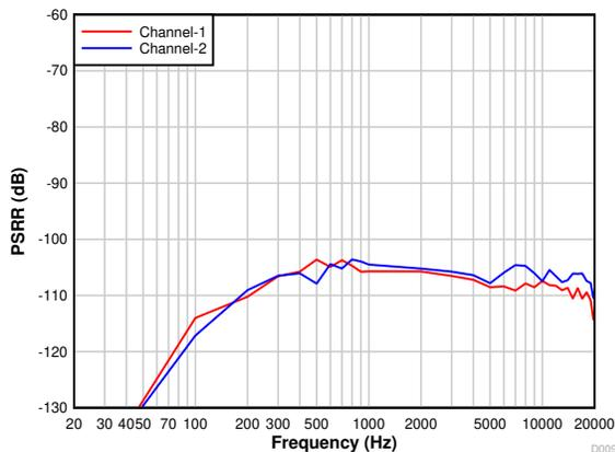
Figure 7-12. Power-Supply Rejection Ratio vs Ripple Frequency With 100-mV<sub>PP</sub> Amplitude
