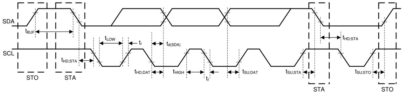
图 7-1. I<sup>2</sup>C Interface Timing Diagram
