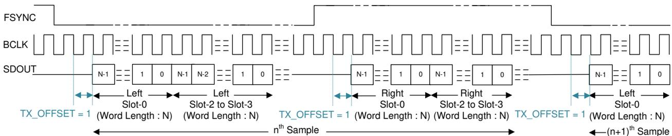
图 8-6. I<sup>2</sup>S Protocol Timing (TX\_OFFSET = 1)
