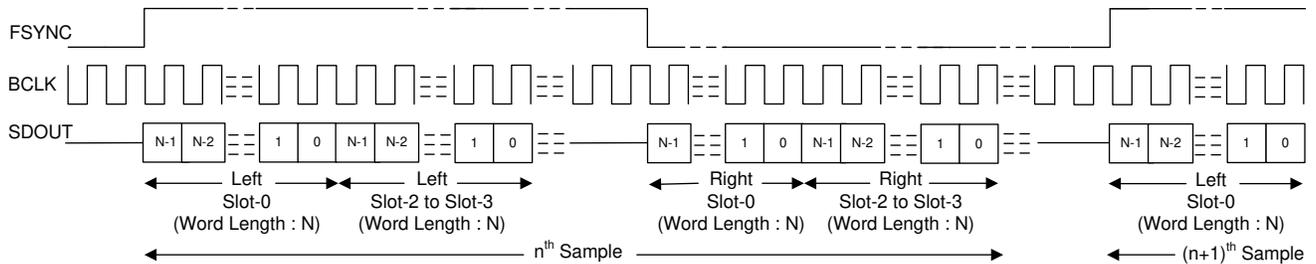
图 8-9. LJ Mode Standard Protocol Timing (TX\_OFFSET = 0)
