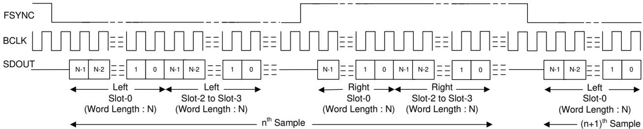
图 8-5. I<sup>2</sup>S Mode Standard Protocol Timing (TX\_OFFSET = 0)
