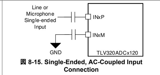
The device allows for flexibility in choosing the typical input impedance on INxP or INxM from 2.5 k $\Omega$  (default), 10 k $\Omega$ , and 20 k $\Omega$  based on the input source impedance. The higher input impedance results in slightly higher noise or lower dynamic range. 表 8-9 lists the configuration register settings for the input impedance for the record channel.
