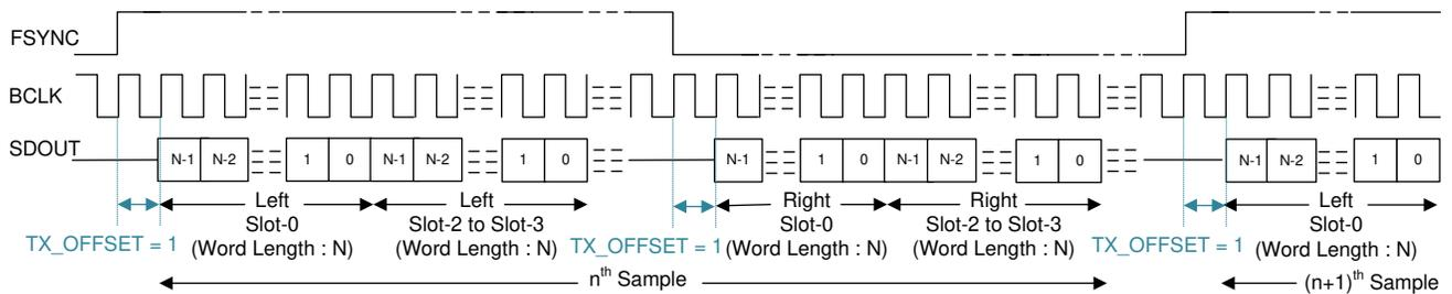
图 8-12. LJ Protocol Timing (TX\_OFFSET = 1 and BCLK\_POL = 1)
