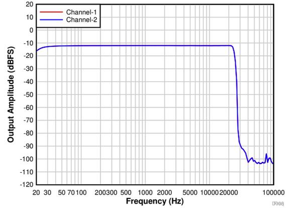
Figure 7-11. Frequency Response With a -12-dBr Input
