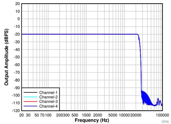
Figure 7-19. PDM Input Frequency Response With a -20-dBr Input
