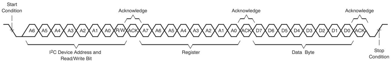
**Figure 8-67. I<sup>2</sup>C Single-Byte Write Transfer**
