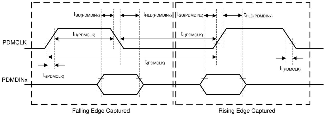
**图 7-3. PDM Digital Microphone Interface Timing Diagram**
