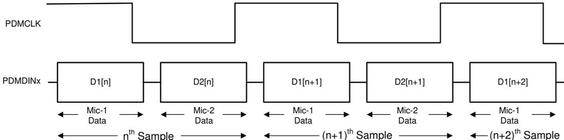
shows the digital PDM microphone interface timing diagram.
