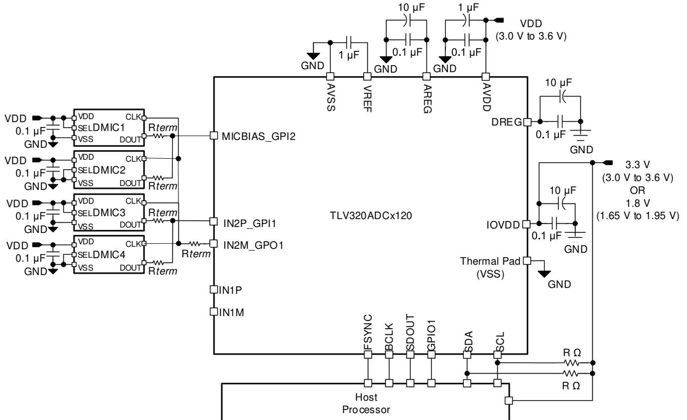
图 9-4. Four-Channel Digital PDM Microphone Recording Diagram
