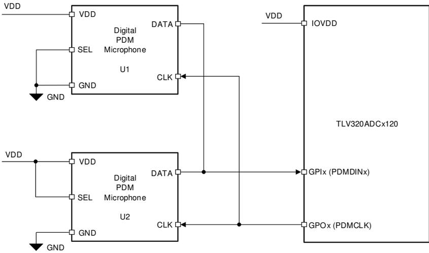
shows a connection diagram of the digital PDM microphones.
