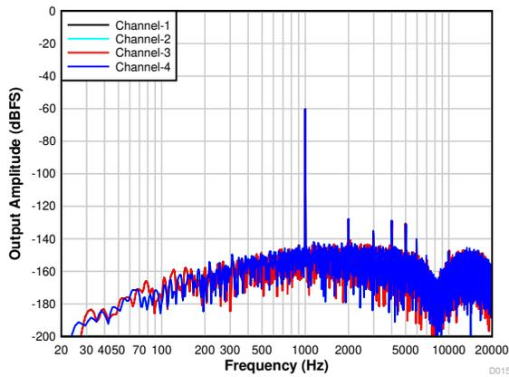
Figure 7-18. PDM Input FFT With a -60-dBr Input
