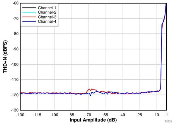
Figure 7-16. PDM Input THD+N vs Input Amplitude
