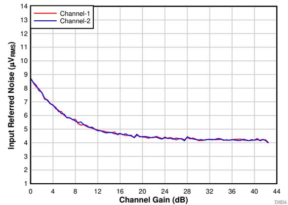
7-9. Input-Referred Noise vs Channel Gain
