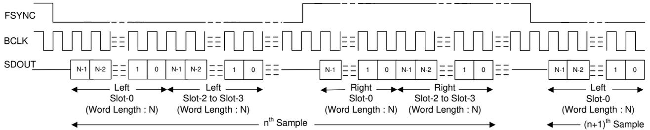
图 8-8. I²S Protocol Timing (TX\_OFFSET = 0 and BCLK\_POL = 1)
