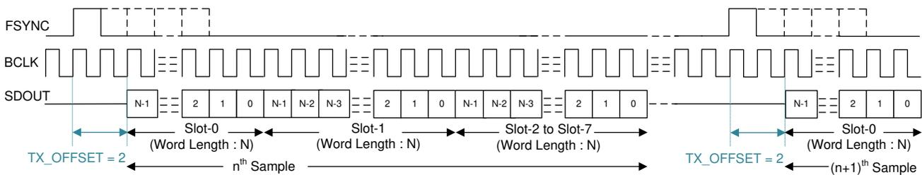
**图 8-2. TDM Mode Protocol Timing (TX\_OFFSET = 2)**
