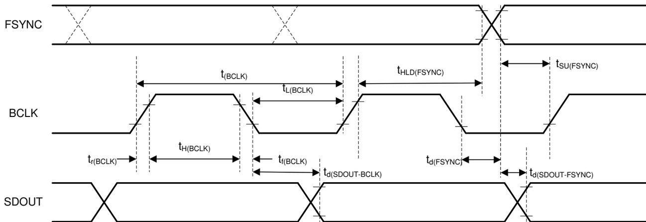
图 7-2. TDM (With BCLK\_POL = 1), I<sup>2</sup>S, and LJ Interface Timing Diagram
