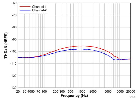
7-8. THD+N vs Input Frequency With a  $-1\text{-dBr}$  Input
