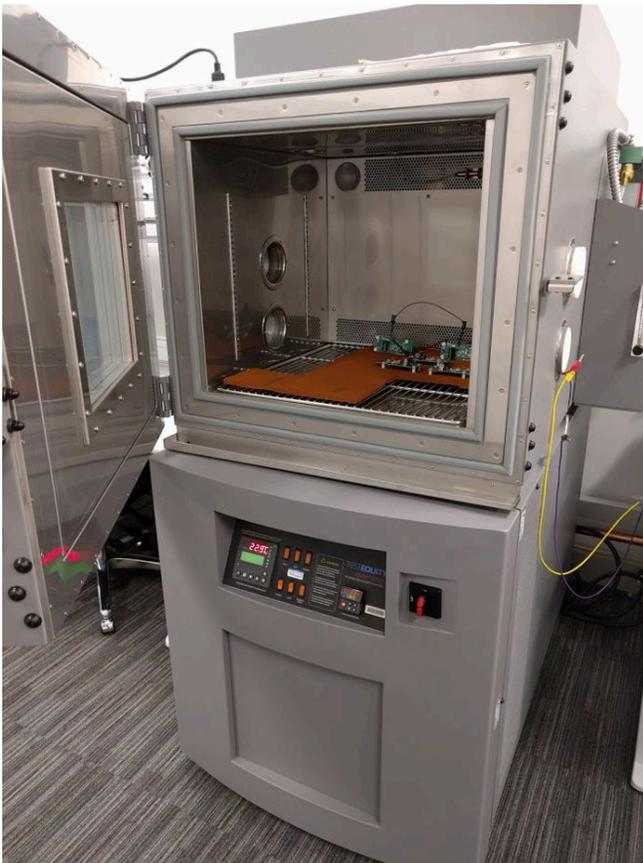
☒ 26. Temperature and Humidity Test Setup
