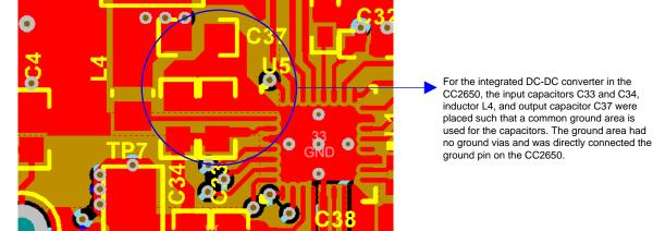
図 41. DC/DC Routing Guidelines
