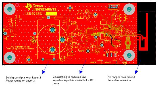
**2** 40. Low-Power Carbon Monoxide Sensor Reference Design Layout Guidelines
