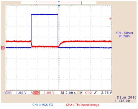
図 8. Sensor in Short-Circuit
