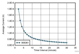
2 33. Combined Standby and Test State Average Current versus Timer Interval
