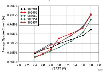
図 28. Standby State Current Consumption Across System Voltage
