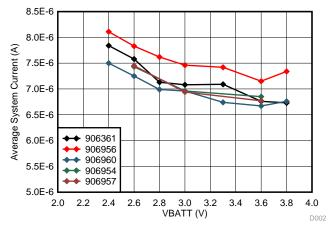
図 31. Pre-Alarm State Current Consumption Across System Voltage
