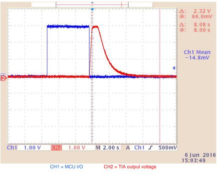
**I 5. Normal Sensor Response to Test Current**
