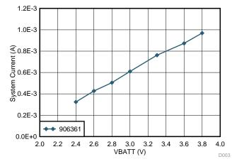
図 32. Alarm State Current Consumption Across System Voltage
