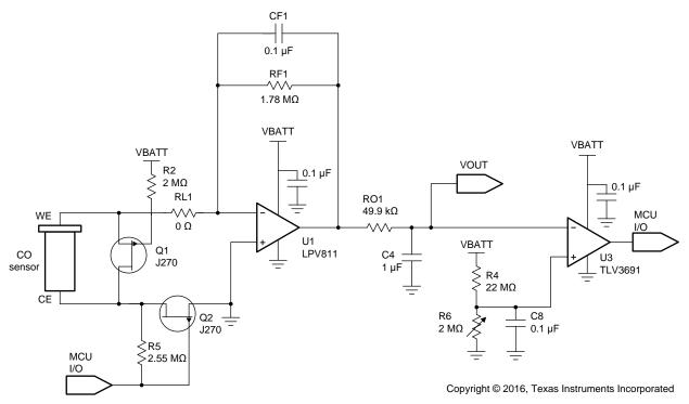
**I** 9. CO Sensor Analog Signal Path Schematic
