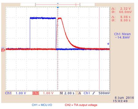
☑ 6. Normal Sensor Response to Test Current (With CO Gas)
