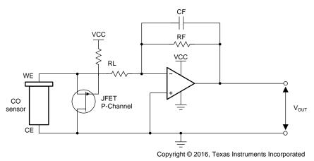
4. Sensor Anti-Polarization Technique Using P-Channel JFET
