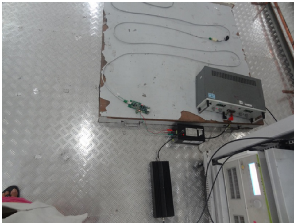
☒ 23. TIDA-00928 Board Testing on Communication Cable With CDN
