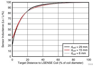
$\boxtimes$  7. Sensor Inductance versus Target Distance L<sub>SENSE</sub> Inductance (L<sub>s</sub>) Varied, L<sub>REF</sub> Inductance (L<sub>r</sub>) Fixed
