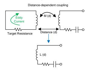
6. Electrical Model of Series Inductive Sensor
