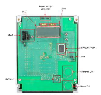
☑ 44. TIDA-01377 One-Sense-Coil Variant PCB With Components Highlighted—Top View
