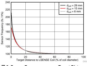
$\label{eq:sense} \boxed{\ensuremath{\mathbb{Z}}} \ 8. \ Sensor \ Frequency \ versus \ Target \ Distance \\ L_{\text{SENSE}} \ Frequency \ (f_s) \ Varied, \ L_{\text{REF}} \ Frequency \ (f_r) \ Fixed \\ \hline$
