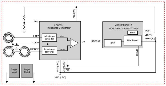
2. System Block Diagram—Two-Sense-Coil Variant
