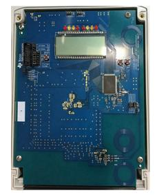
☑ 45. TIDA-01377 PCB Two-Sense-Coil Variant Top View
