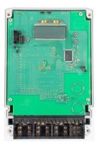
☑ 43. TIDA-01377 PCB One-Sense-Coil Variant Top View
