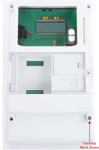
24. Terminal Block Cover Fully Screwed onto Main Cover
