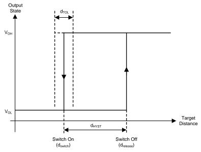
図 14. Switching Distance Hysteresis and Threshold Tolerance
