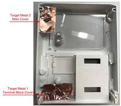
31. Target Metal Placement on Case
