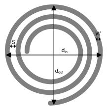
**図 10. Example PCB Coil Geometry**
