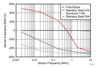
☑ 35. Sensor Inductance Shift versus Sensor Frequency for Conductive Target Metals
