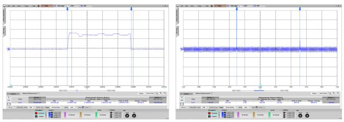
☑ 52. Average Current Consumption: LDC0851 Enabled, Two-Sense-Coil Implementation
