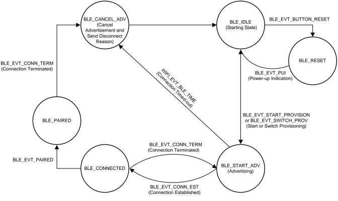
**7** shows the state machine implemented by the task that is dedicated to provisioning over BLE.
