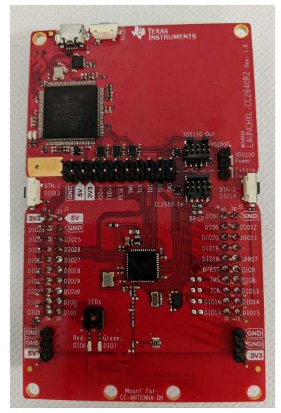
図 12. CC2640R2F LaunchPad<sup>™</sup> Configuration
