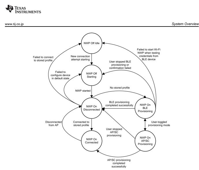
☑ 5. Network-Connection Management-Thread Flow Diagram
