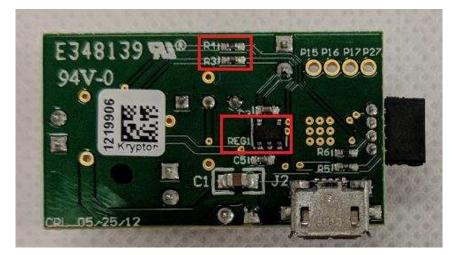
23. Back of DRV8837EVM With Components To Remove Highlighted
