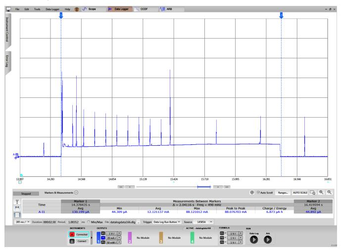
図 26. CC3220 Current Consumption During Lock and Unlock Cycle
