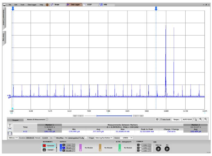
図 25. CC3220S Current Consumption Versus Time While in Idle Connected Mode With 400-ms LSI
