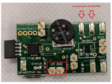
図 14. J1 and IN1/IN2 Highlighted on Front of DRV8837EVM
