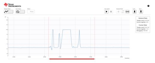
図 31. Collector Current Consumption for Transmission of 150-Byte Data
