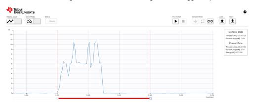
27. Sensor Current Consumption for Reception of 1-Byte Data
