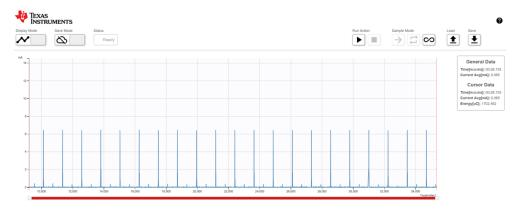
In 19. Sensor Current Consumption for a Beacon Interval of 1.23 s
