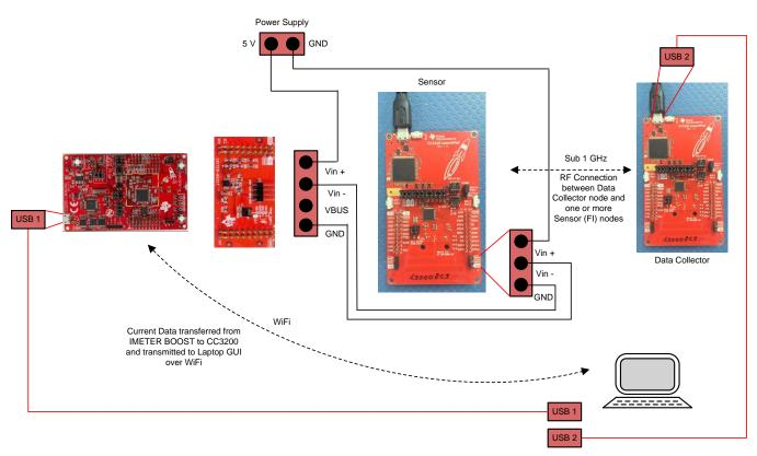
図 17. TIDA-00816 Test Setup for Current Measurement
