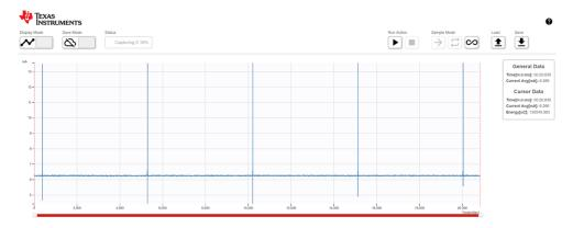
21. Collector Current Consumption for a Beacon Interval of 4.92 s
