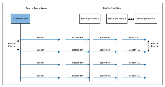
All Sensor (FI) nodes connected to the PAN will track the beacon and enable RX just before the start of the Beacon.
