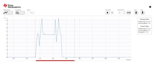
28. Sensor current consumption for reception of 150-Byte Data
