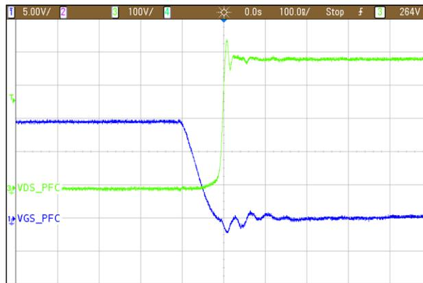
図 12. PFC MOSFET Turnoff Waveform at 230 V
