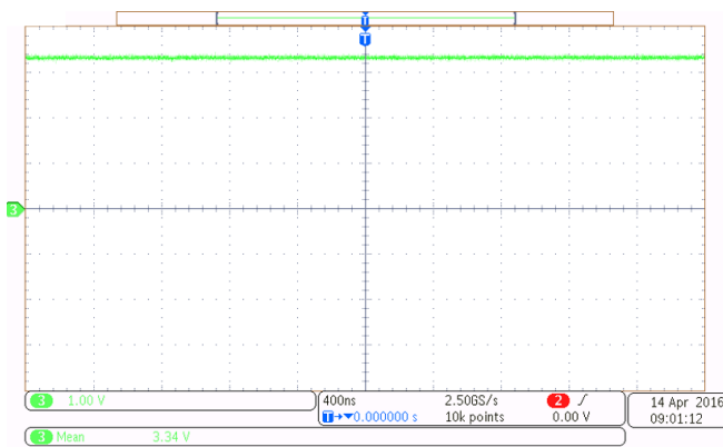
☒ 32. 3.3-V Rail Generated Using REF2033
